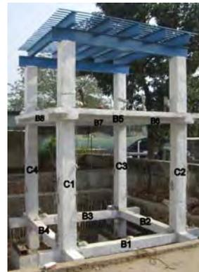
Figure 5 (a). Time-temperature plots for the compartment fire. (b). Sub-assembly nomenclature.
