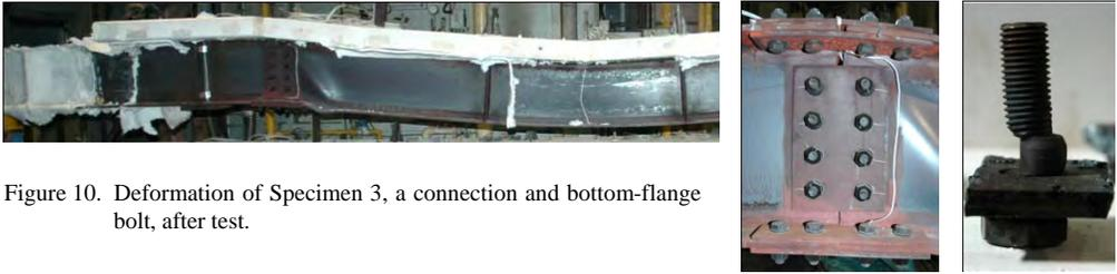
Figure 10. Deformation of Specimen 3, a connection and bottom-flange bolt, after test.
