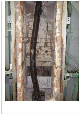
Figure 7. Failure mode of the concrete filled elliptical column.
