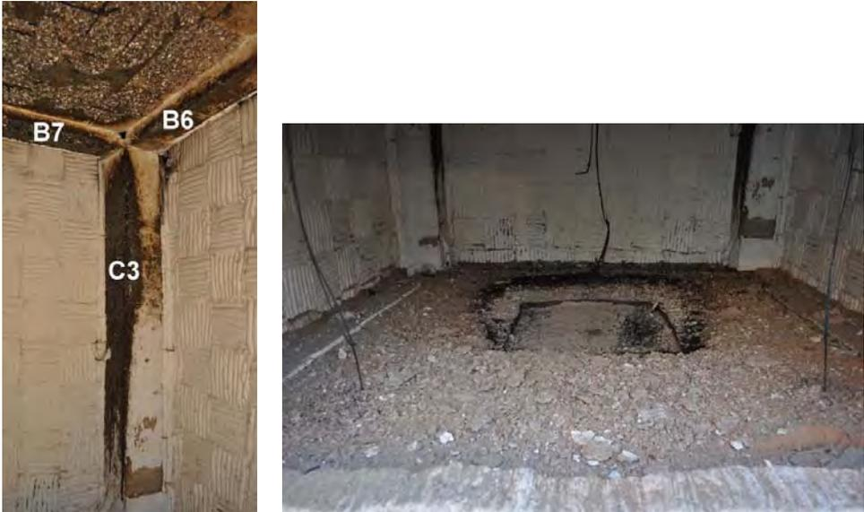
Figure 6 (a). Frame sub-assembly after the fire test (b). Extent of spalling (debris) on compartment floor.
