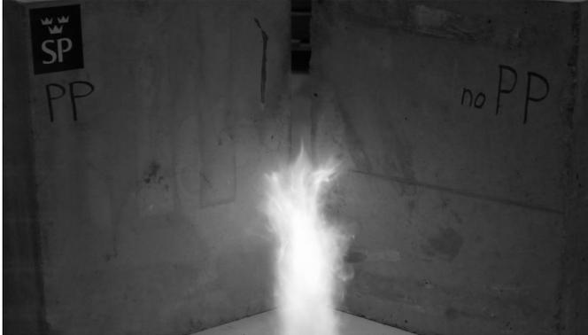
Figure 2. First heating no spalling. In the slab on the left side PP fibres were included.
