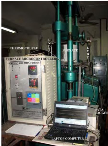
Figure 2. Rebar test at elevated temperature in progress
