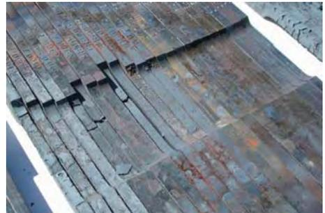
Figure 11. Coupons after creep testing
