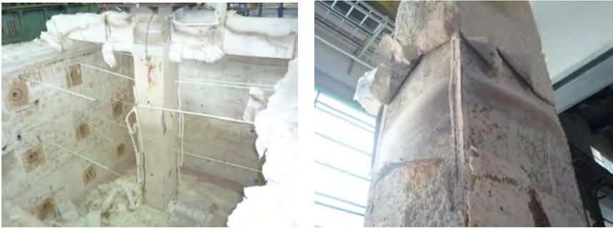
Figure 8. Appearance of Spec. CFBC-2 at conclusion of the test.
