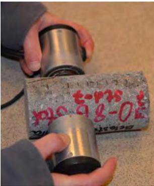
Figure 2. Photo showing an example of ultrasonic pulse velocity measurements on concrete cores [12].
