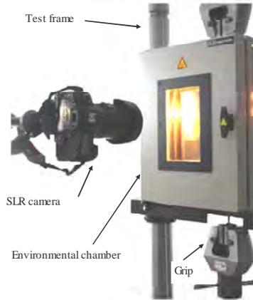
Figure 2. Test setup and digital SLR camera used for DIC analysis.
