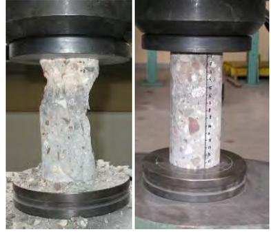
Figure 9. Point-by-point analyses of concrete on cores drilled from thermally damaged HPC's slab.
