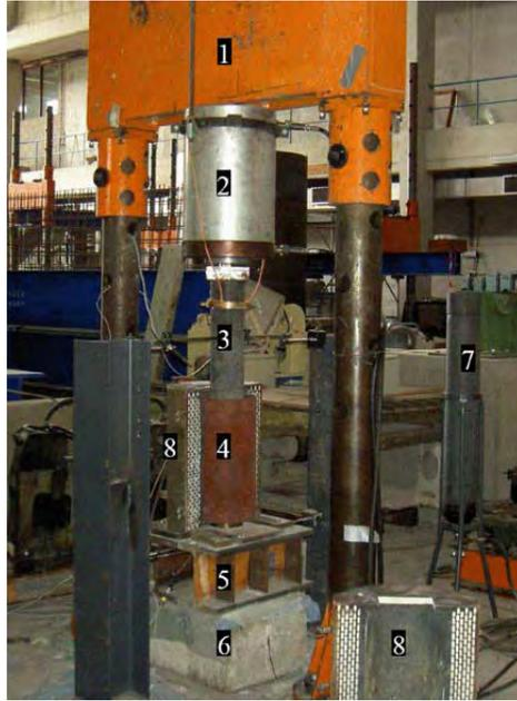
Figure 1. Test setup: (1) loading frame, (2) hydraulic jack, (3) series of X105 Cr Mo 17 steel cylinders, (4) tube around concrete specimen, (5) HE 200 M profiles, (6) concrete block, (7) accumulator, (8) oven.
