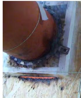
Figure 7. Failure in sealed penetration junction
