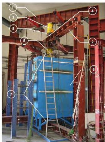
Figure 1. Experimental set-up for fire resistance tests on columns
