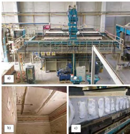
Figure 2. a) General view of the experimental setup. b) Inside the furnace. c) Voids infilling.
