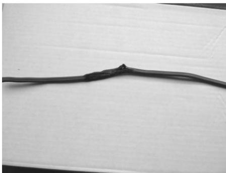
Figure 8. Crushed alarm cabling (courtesy FPANZ).
