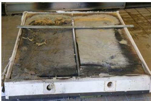
Figure 10. Hot air stream may cause local decompositions of the material (left side). Photo taken after fire test SP Wood Technology
