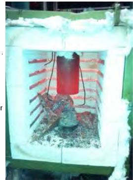
Figure 3. (a) Experimental setup for the measurement of in-situ compressive strength of geopolymer and OPC concrete samples. (b) Inside view of kiln with stainless steel cylinders on top and bottom of concrete cylinder.
