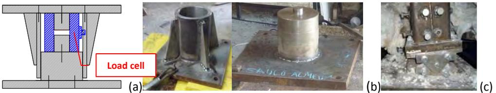
Figure 2 – (a) Scheme of the device for measuring the restraining forces (b) Fabrication of the device (C) column's pin-ended support
