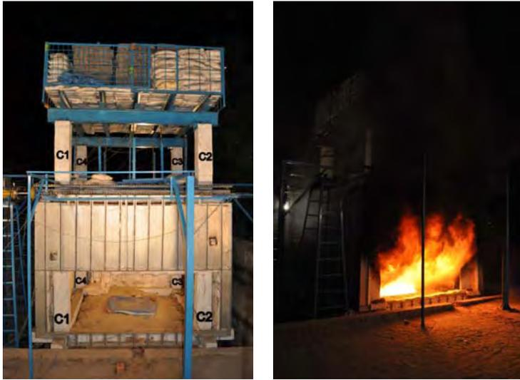
Figure 3 a). Pre-loaded frame before fire b).Fire test.
