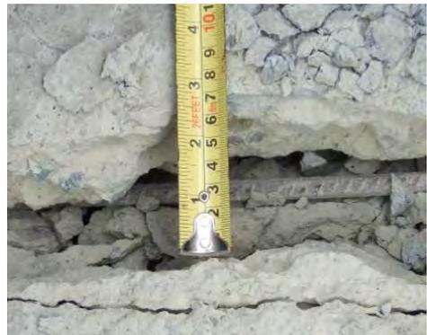
Figure 4. Full depth cracking of the slab after test.
