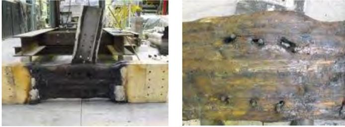
Figure 6. View of specimen B1 after fire test.
