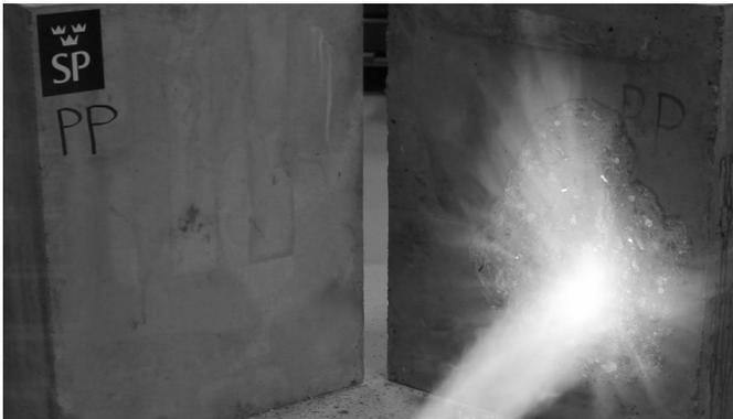
Figure 3. Second heating severe spalling caused by restraint of cold concrete. Note the cracking and moisture flow out from the edge of the spalled concrete.
