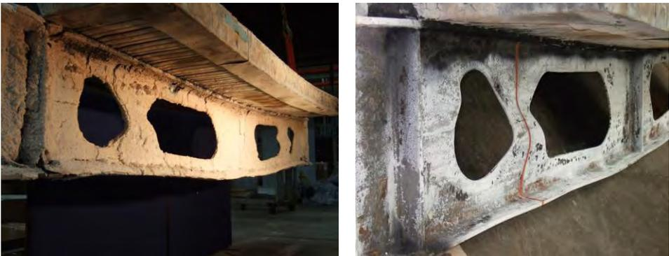
Figure 5: Protected Cellular Beam 2 after the test
