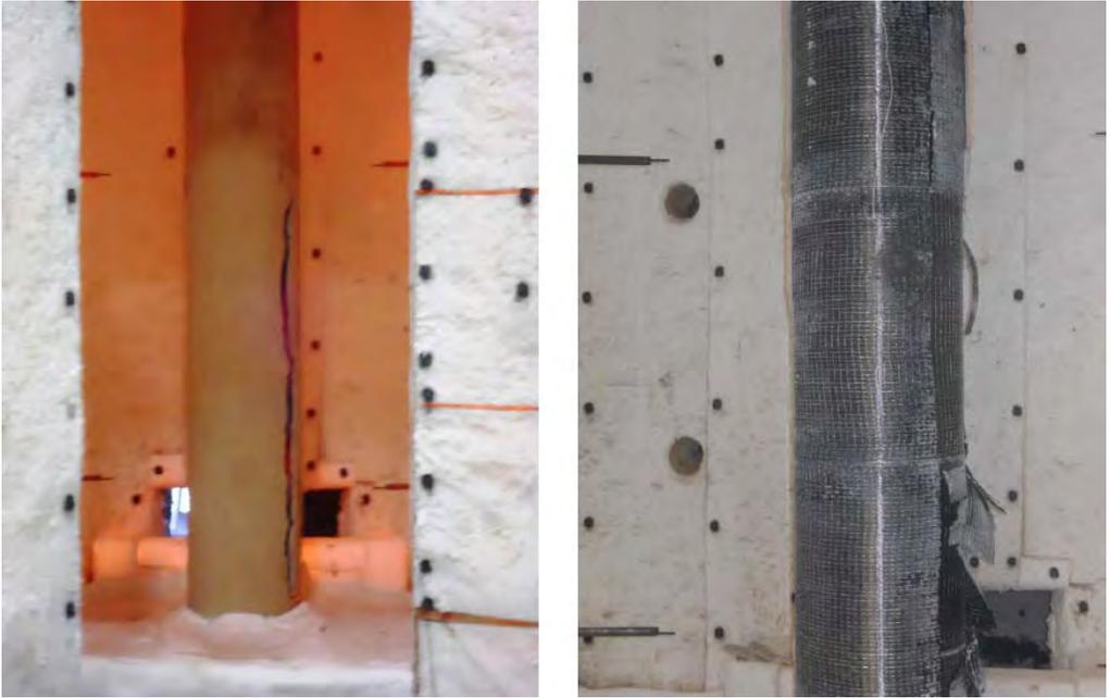
Figure 6. Circular column after fire testing.
