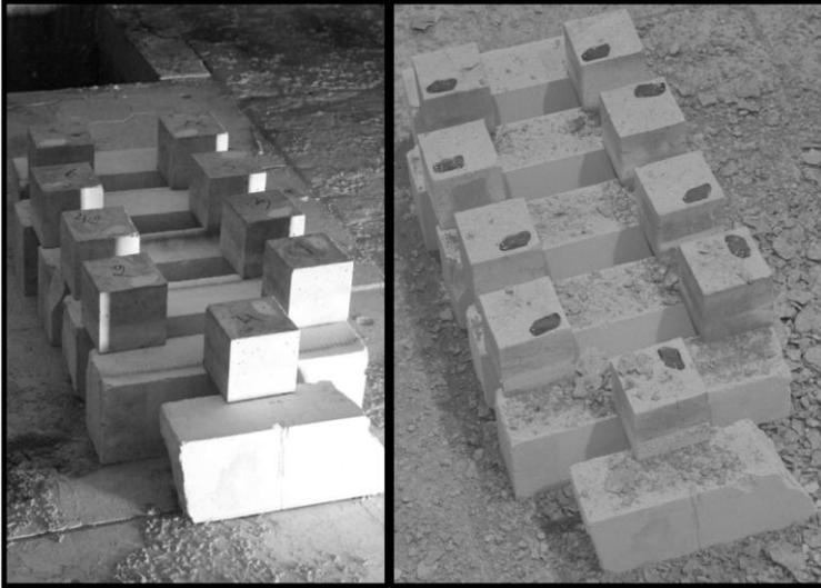
*Figure 4 Before and after a fire test in a horizontal furnace. Non of the fire tested cubes spalled but spalled material from the corresponding large slabs used as a roof during the fire test can be seen around the cubes after the fire test.*
