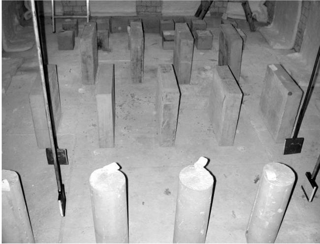
*Figure 5 Small unloaded test specimens made of tunnel concrete in fire testing furnace before fire test.*
