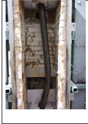
Figure 4. Failure mode of elliptical hollow column.
