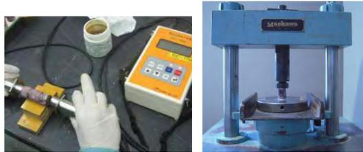
a) UPV test      b) Compressive strength test
