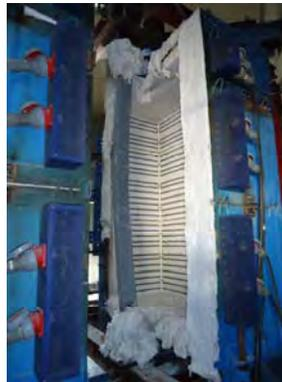
Figure 14. I - cross-section column inside the furnace after test
