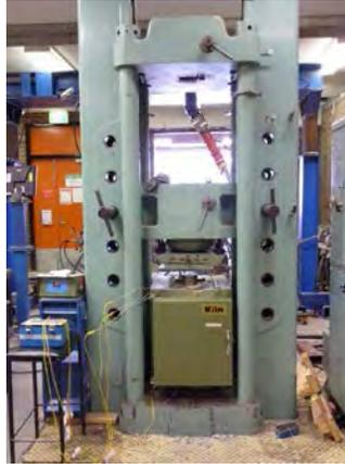
Figure 1. Experimental setup for compression and thermal expansion tests of concrete cylinders at elevated temperatures.
