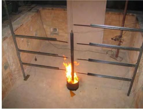
Figure 6. Instrumentation set-up used to measure temperatures at different heights of a pool fire of diameter of 300 mm which engulfs a steel circular column 1500 mm high and of diameter 60.3 mm.
