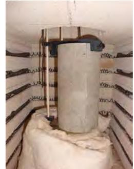
Figure 2. (a) Experimental setup for the measurement of thermal expansion of geopolymer and OPC concrete samples. (b) Inside view of kiln with concrete cylinder and ceramic rod.
