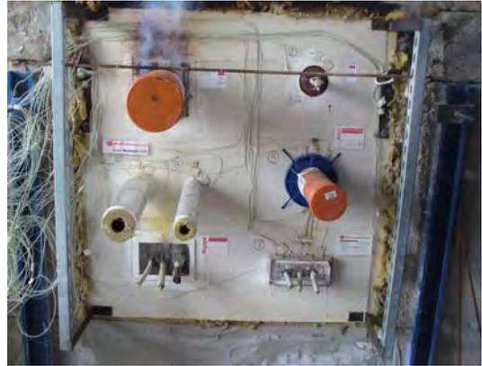
Figure 5. Small scale fire tests assembly (setup 2 - EI90)
