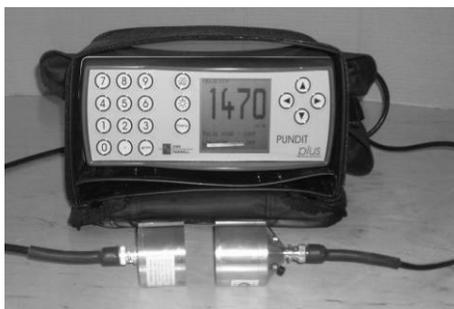
Figure 1. PUNDIT plus ultrasonic test equipment.
