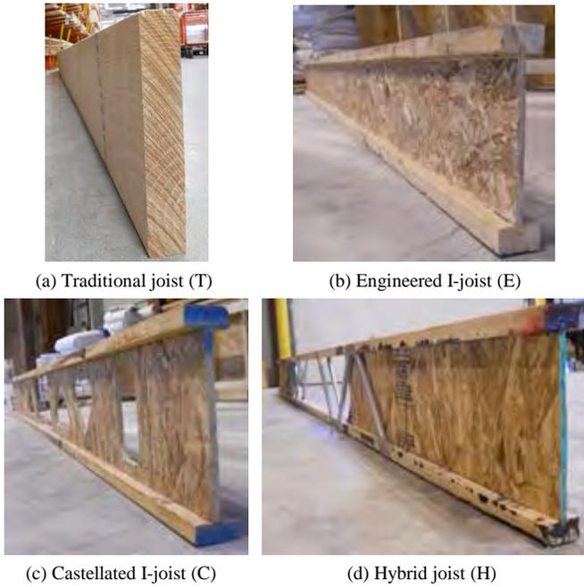
Figure 1. Typical traditional and engineered wood joists considered in fire resistance tests.
