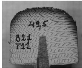
Figure 10: Simulation results for bending resistance (curves GtA and GtF) and test results (left). Cross-section of the exposed flange of the burnt but intact finger joint of test GtF 2 after the test.
