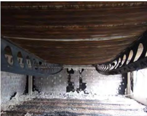
Figure 3. Deformed state of the internal beams after test.
