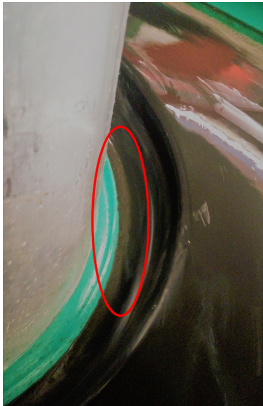
Figure B.5: Slow-moving bed of sand near the column in 20% diluted sludge.
