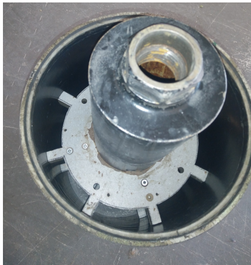
Figure B.1: Connection of cylinder to drill with two plates.
