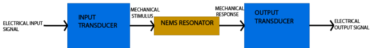
Figure 1.1: Transduction mechanism in a nanoresonator. Adapted from [2]
