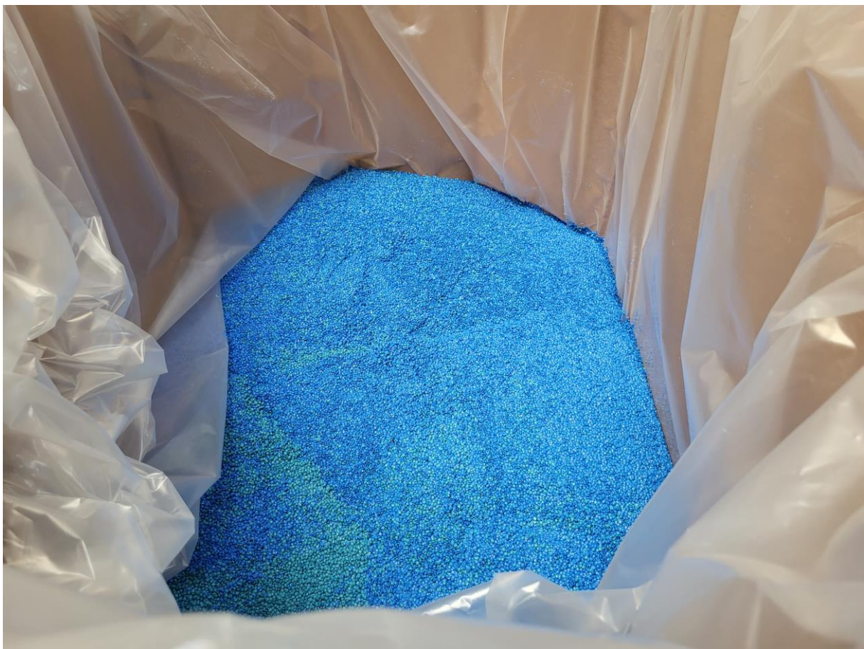
Figure 9. High-grade medical GC rPP raw material pellets made by GreenCycl out of used blue wrapping paper. Photo by B. van Straten.
