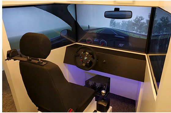
Fig. 2. The fixed-based driving simulator.
