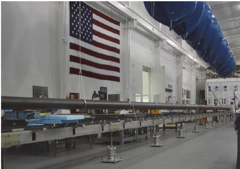
**Figure 6.1:** Deployed stiffness test configuration for the Telescopic Tubular Mast (TTM), Developed by Astro Aerospace, a division of Northrop Grumman Aerospace Systems[13]
