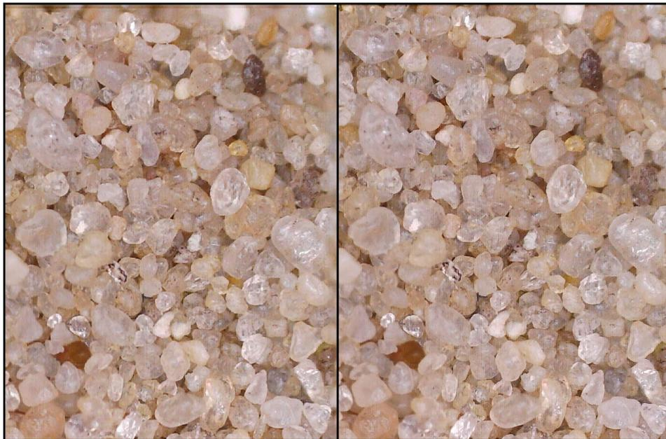
**Figure 3.10:** Close-up of the two focus stacking methods. On the left using Adobe Photoshop and on the right using Helicon Focus 8. Note the lines on top of the left image and the increased blur on the right of the left image.
