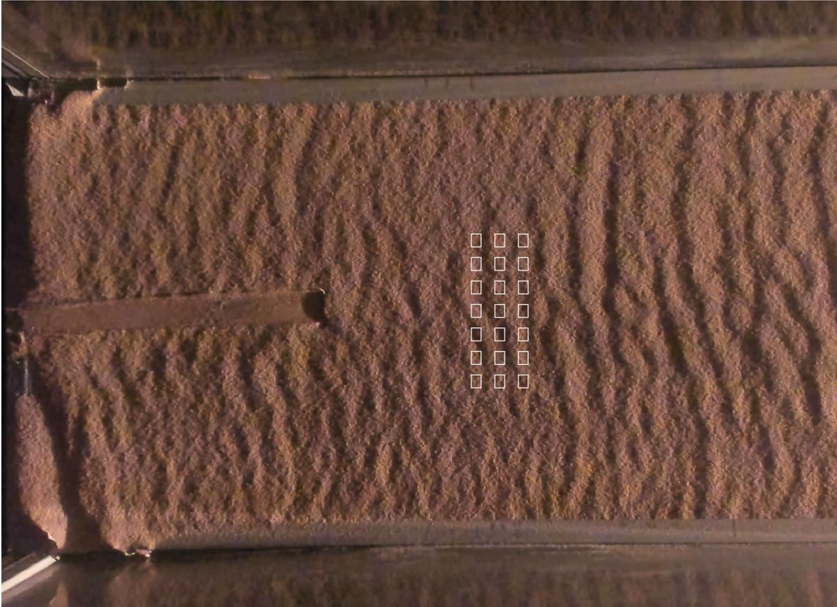
**Figure A.1:** In white, grid of images taken using the microscope. The images were taken at 2 *cm* intervals, with the size of each image encompassing approximately 1.1 by 0.8 *cm* of the sandbed. Top view, the flow direction is right to left. On the left, the imprint left in the sand is that of the sand trap.
