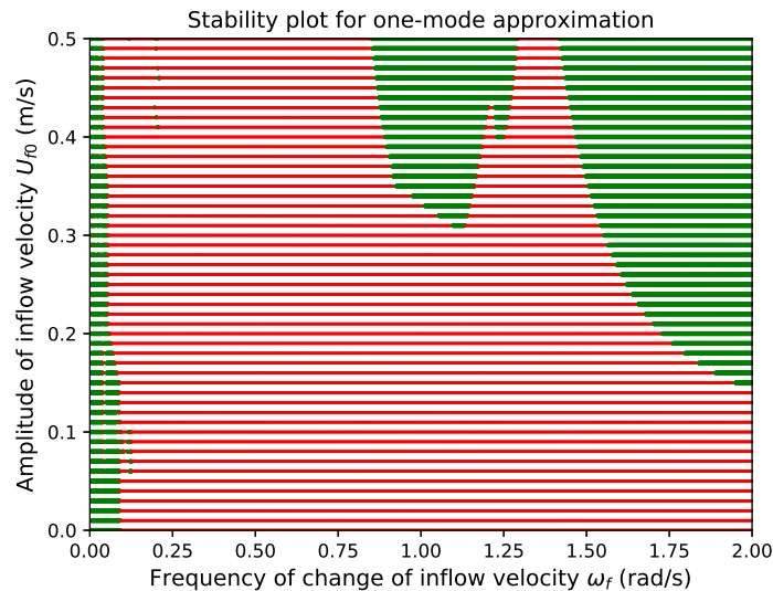
Figure 6.1: Stability plot for the pipe using the one-mode approximation for different combinations of U_{f0} and \omega_f . Combinations that yield a stable value plotted in green, combinations that yield an unstable value plotted in red.
