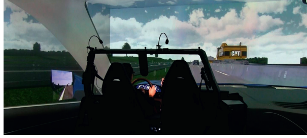
FIGURE 1: The hexapod simulator during a takeover scenario. The participant has regained manual control and made a lane change to the left lane. Roadworks can be seen behind the wall in the right lane.
