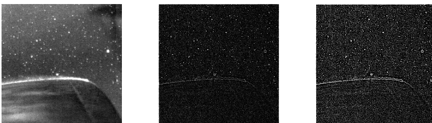
Figure 4.2 This example shows the original image at left and two results from a Laplacian kernel; the K_{LA} (center) and K_{LS} (right). The gradients in the image are captured.
