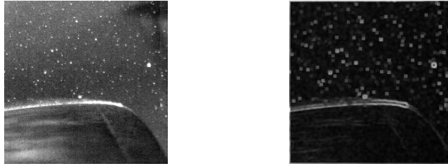
Figure 4.4 The standard deviation gives a good indication of activity in the image and yields a result that is close to the Sobel filter, but the result is less sharp.
