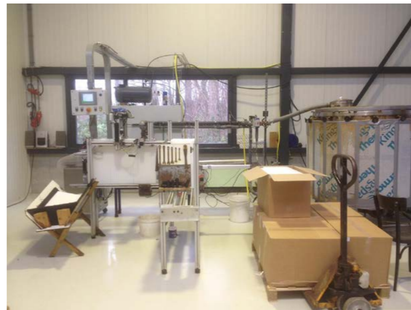
Encapsulation space: 40 PCM is pumped around an machinally fills the HDPE containers, then it falls in the 'crib' before it is tested on leakage (not in photograph)
