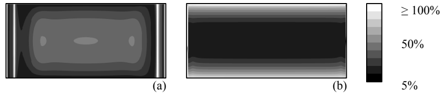
Figure 9. Comparison of the strain maps obtained from simulated phase maps and the finite element simulated strain. Without the sensitivity vector correction. (a) Longitudinal and (b) tangential strain.
