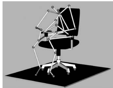
Figure7- 5 Experiment in office chair design using posture prediction technology
