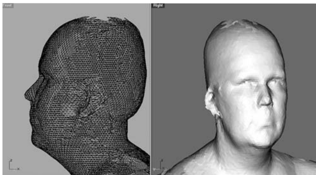
Figure 2-1 Incomplete meshes on the top of the head and the ears area of the sample acquired by 3D surface anthropometry
