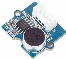
Figure 3.3: Sound intensity sensor [11].
