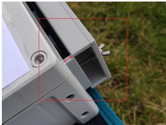
Figure 3.27: Sensor box rain protection open vs close.
