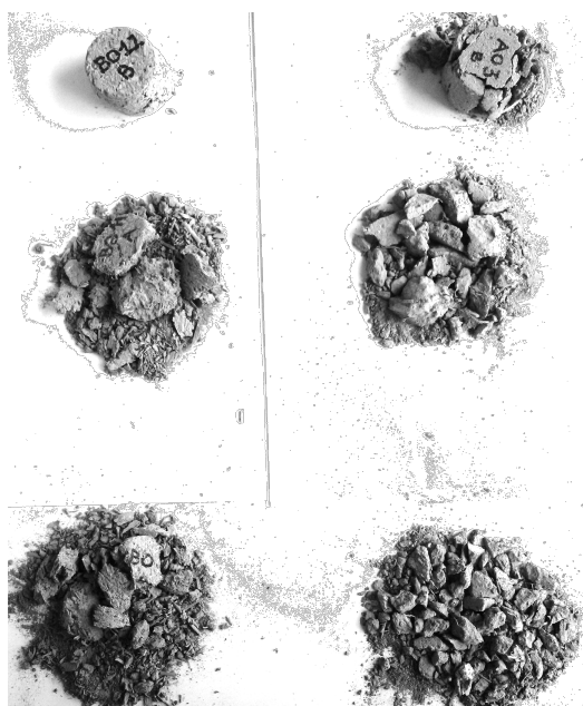
Figure 4.8: Typical post-mortem comparison of Type A (right) and Type B(left) for static test (first row), intermediate strain rate test (second row) and split Hopkinson bar test (third row)
