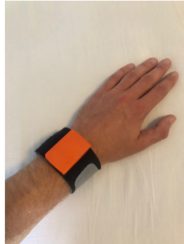
Figure 1-1: Xsens [1] MTw Awinda wearable MEMS IMU containing a gyroscope and an accelerometer. Arm for scale.
