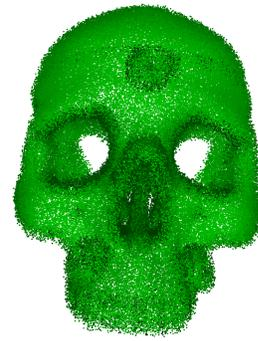
Figure 5: Simulated front-view depth sensor point cloud with random noise added
