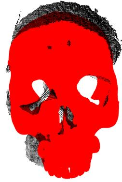
Figure 9: FPFH rough alignment with downsampled source and depth sensor data. The black point cloud is the depth sensor data, the red point cloud is the pre-operative model.
