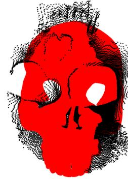
Figure 10: PCA rough alignment on real depth sensor data. The black point cloud is the depth sensor data, the red point cloud is the pre-operative model.
