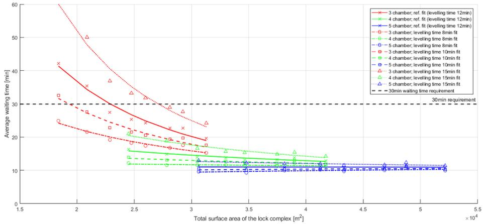
Figure G.4: Average waiting time for the different model variants for varying levelling times at complex G11W5
