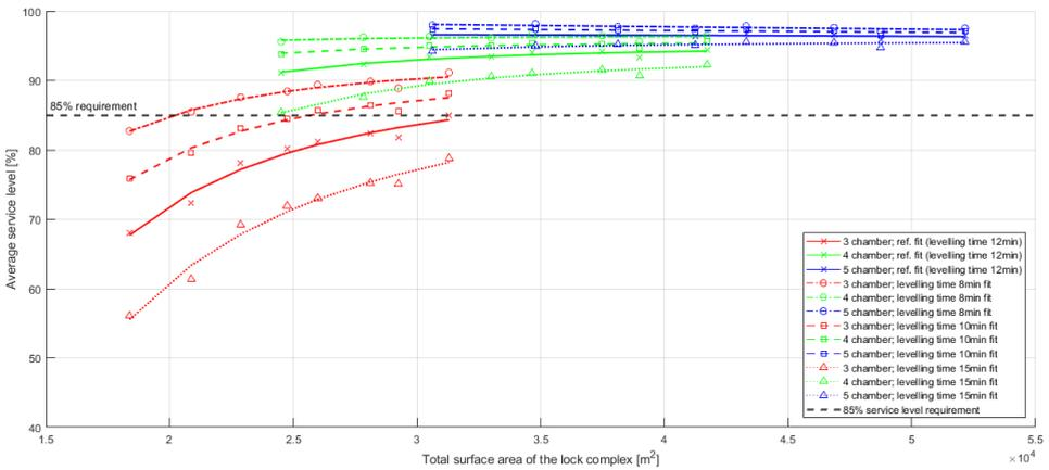
Figure G.5: Average service level for the different model variants for varying levelling times at complex G11W5
