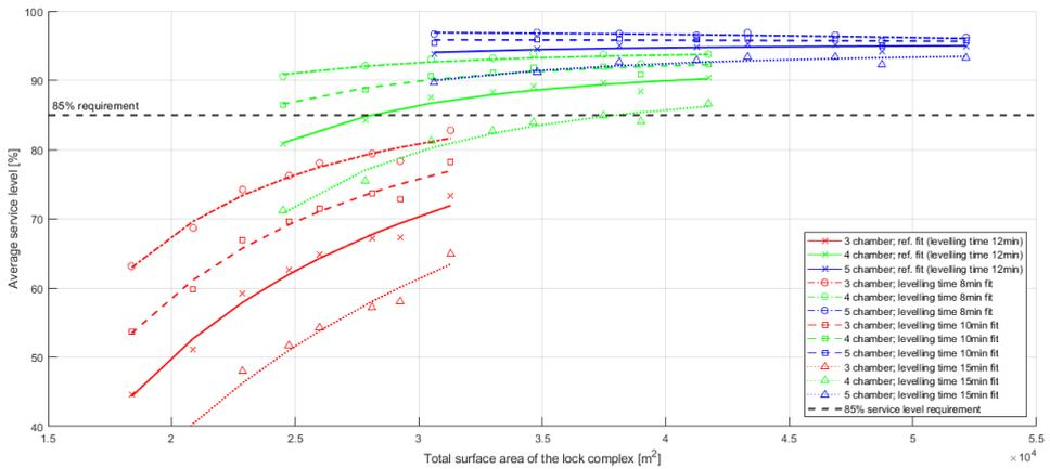
Figure G.3: Service level for the different model variants for varying levelling times at lock complex G11W3
