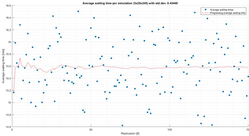
**Figure E.4:** Variation in average waiting time (over four weeks of simulation time) for scenario with four lock chambers (25x330m)
