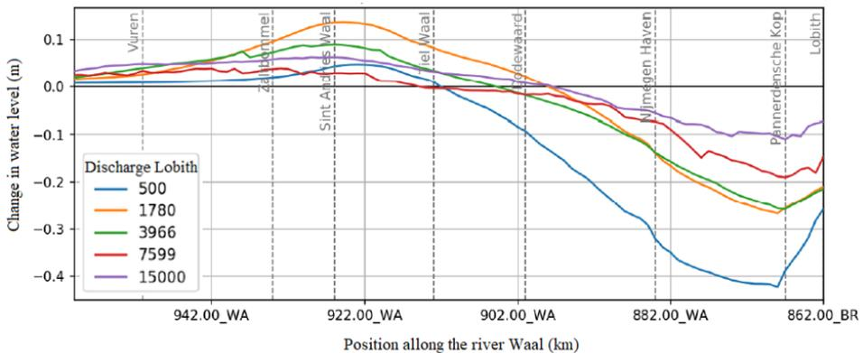
Figure 2.4: Change in water level along the river Waal as a consequence of reach scale bed erosion in 2050 with respect to 2018 (De Jong, 2020b).
