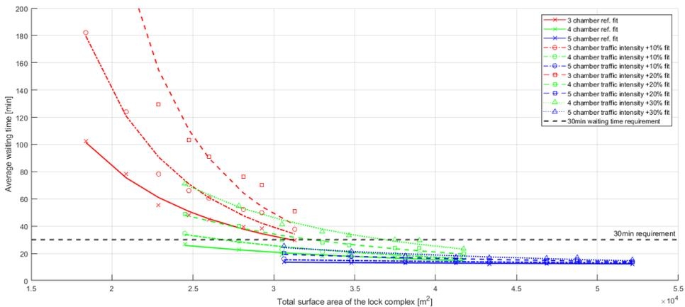
**Figure 5.5:** Average waiting time for all model variants for varying vessel traffic intensities
