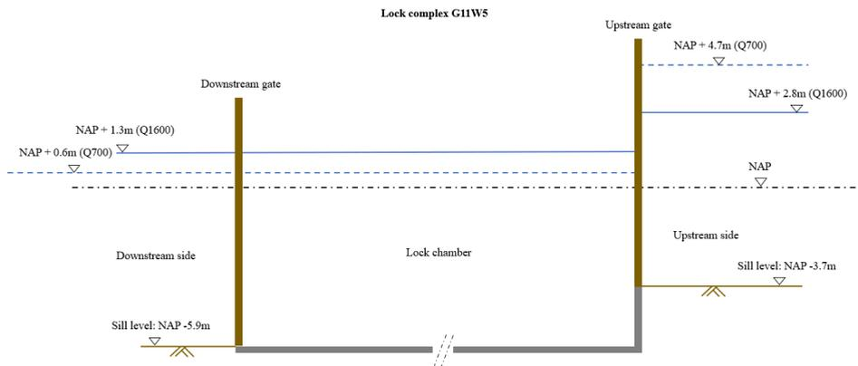
**Figure 4.4:** Longitudinal section of a lock showing normative water levels and sill depths at lock complex G11W5
