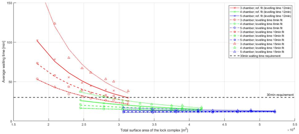
Figure G.2: Average waiting time for the different model variants for varying levelling times at lock complex G11W3
