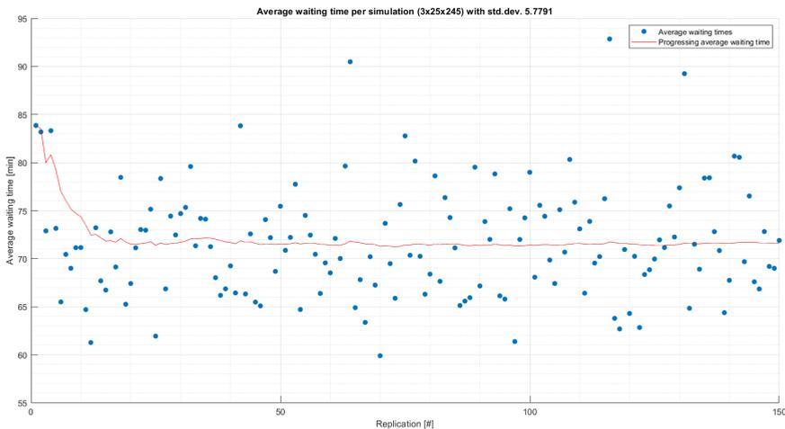
**Figure E.3:** Variation in average waiting time (over four weeks of simulation time) for scenario with three lock chambers (25x245m)
