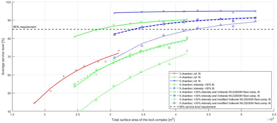
Figure 5.8: Service level for model variants for varying fleet compositions
