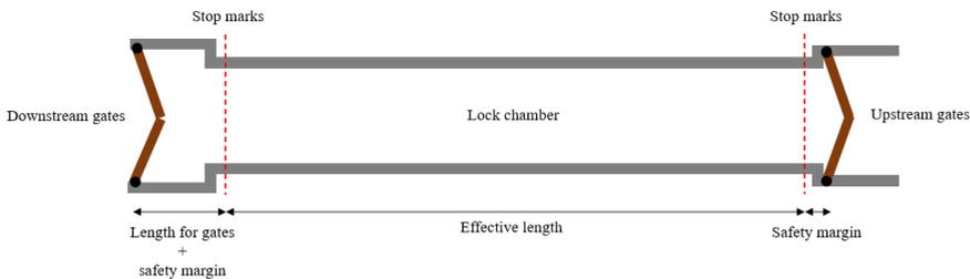
**Figure 4.2:** Top view of a lock and corresponding length definitions
