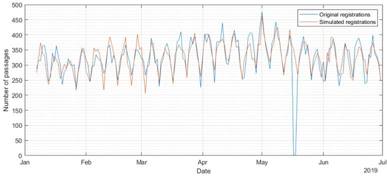
**Figure E.6:** Comparison between original IVS vessel registrations and vessel generation in SIVAK III for the four busiest weeks
