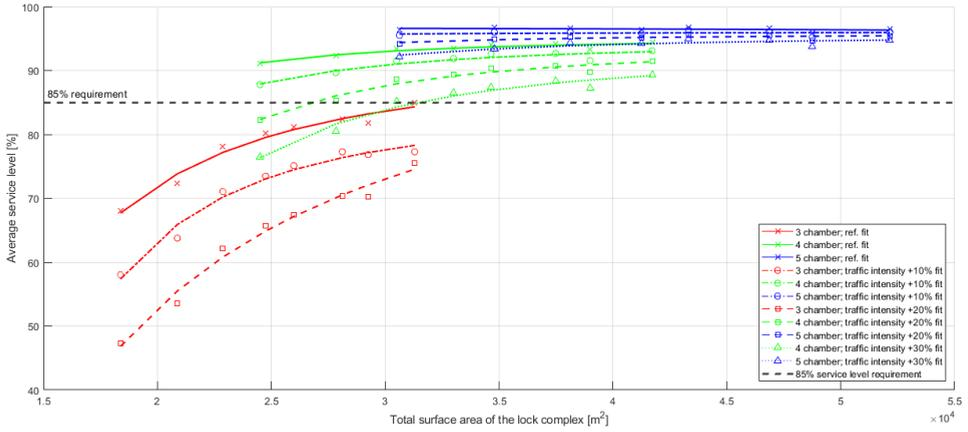
Figure F2: Average service level for all model variants for varying vessel traffic intensities for complex G11W5
