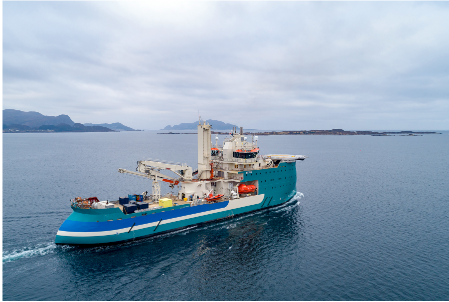
Figure 1.1: Example of a C/SOV. The 'Acta Centaurus' is operated by Acta Marine and features a 120 person accommodation, motion compensated gangway and crane as well as refuelling capacity for smaller CTVs.
