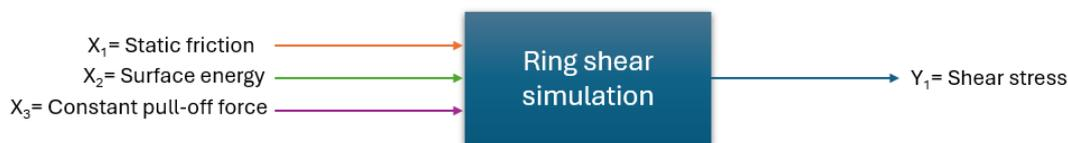
Figure 4.6: Design Of Experiments for sensitivity analysis
