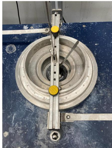
Figure 3.2: Schulze's Ring shear Tester
