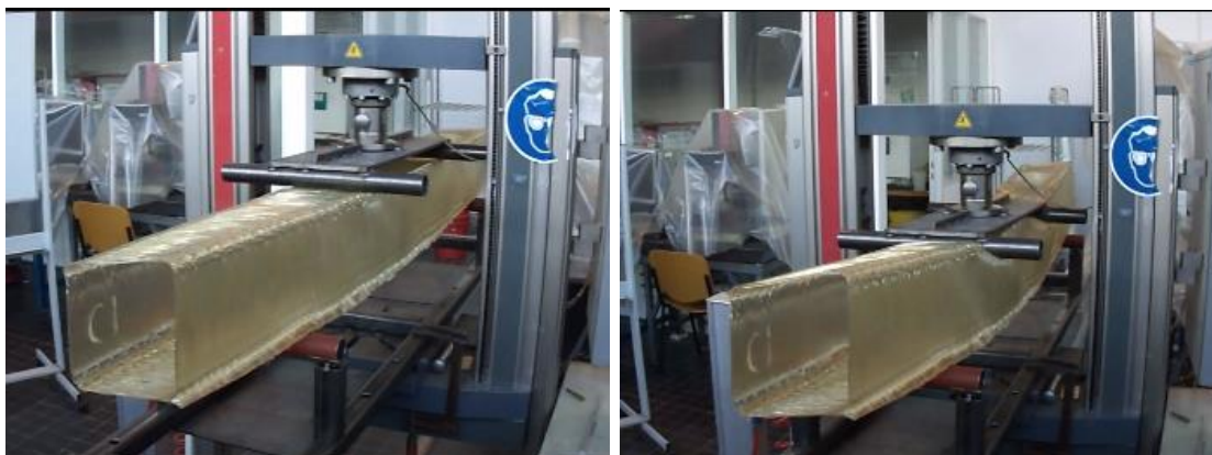
Fig. 139 Testing of block C1, failure probably occurs due to local bending of the top flange or local buckling of the web, around the area where the line load is applied
