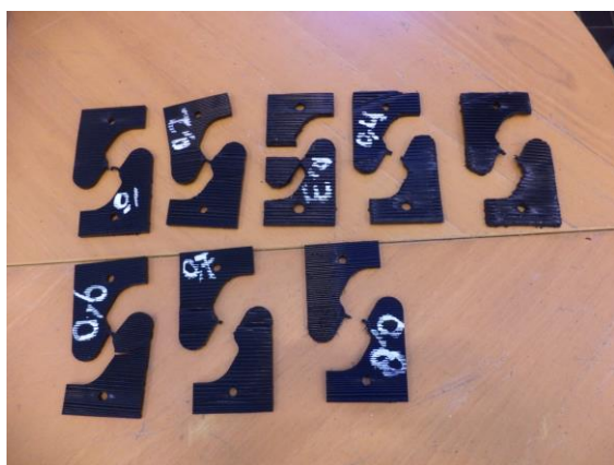
Fig. 51 Shear samples printed in the xz-plane and loaded in shear perpendicular to the grain direction
