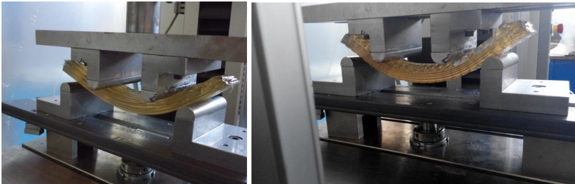
Fig. 132 Left: block type A in bending with its grain in the bending direction. Right: Block type B, which has its grain perpendicular to the direction of bending.
