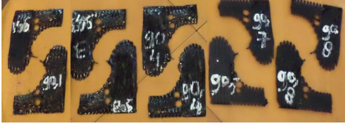
Fig. 58 Tested specimens that are printed within the xy-plane and loaded in shear parallel to the grain
