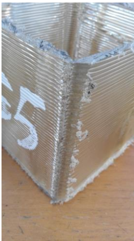
Fig. 114 Weak corner of hollow cube samples at which the samples failed.
