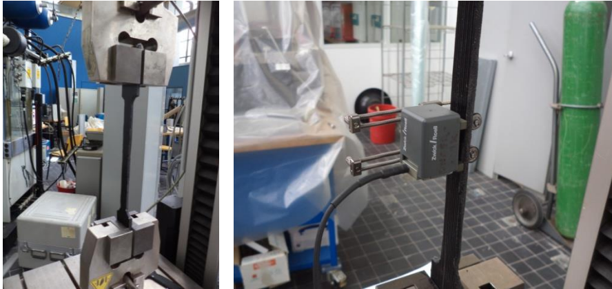
Fig. 103 Sample 500N-test after test performance: no constriction is visible this time
