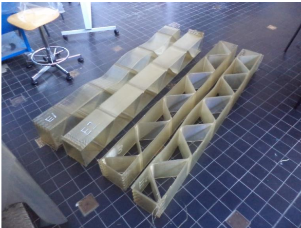
Fig. 128 Beam types E, laid down in the orientation in which they will be tested
