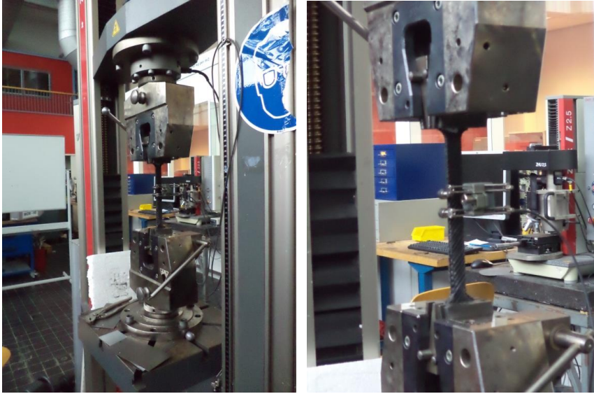
Fig. 72 Test setup for the determination of the Young's moduli
