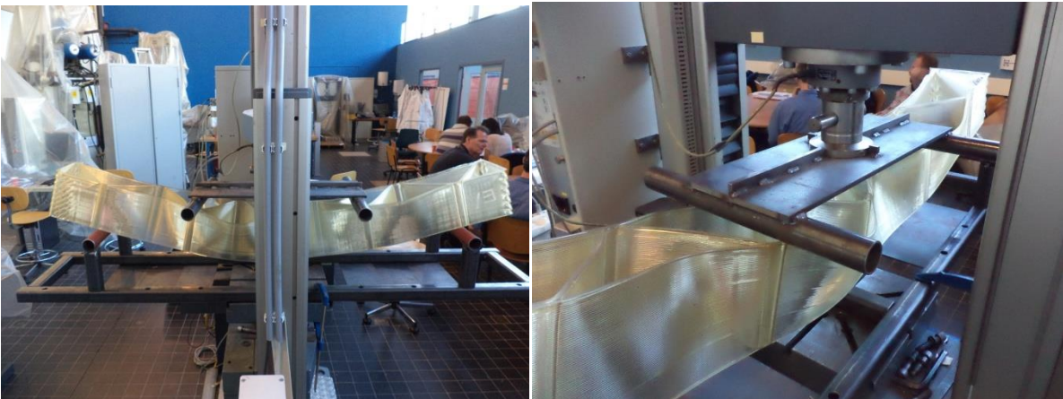
Fig. 142 Testing of blocks E1 and E2, the beam bends as whole but shows local buckling of the webs
