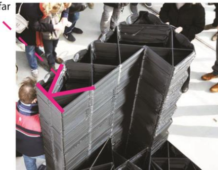
Fig. 29 Within the building project, so far only single lines are printed within the xy-direction. So printing connecting parallel lines in the horizontal plane, like is done for the samples in Figure 27, was a novelty
