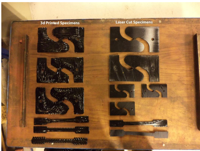
Fig. 37 Left: the specimens that are directly printed within the xy-plane. Right: Specimens that are laser-cut from plates that are printed within the xz-plane.
