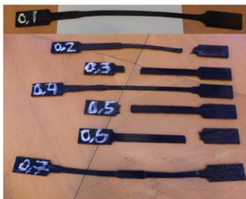
Fig. 41 Left: Specimens printed in the xz-plane and loaded in the grain direction, after they have been tested. Right: Curves of the tests specimens
