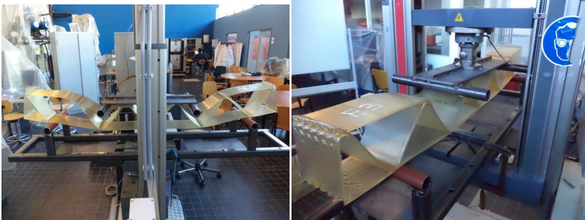
Fig. 143 Testing of blocks E3 and E4, only a small load can be applied due to local bending of the top-flange
