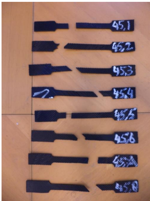
Fig. 43 Left: Samples that are loaded 45 degrees to the grain direction and their curves
