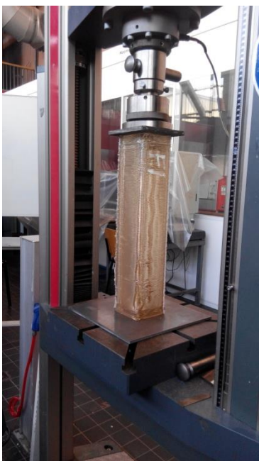
Fig. 112 Test setup – buckling test
