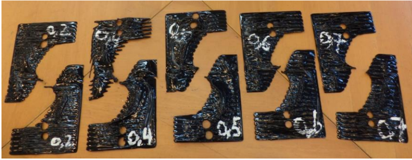
Fig. 56 Test specimens printed within the xy-plane and loaded in shear perpendicular to the grain direction
