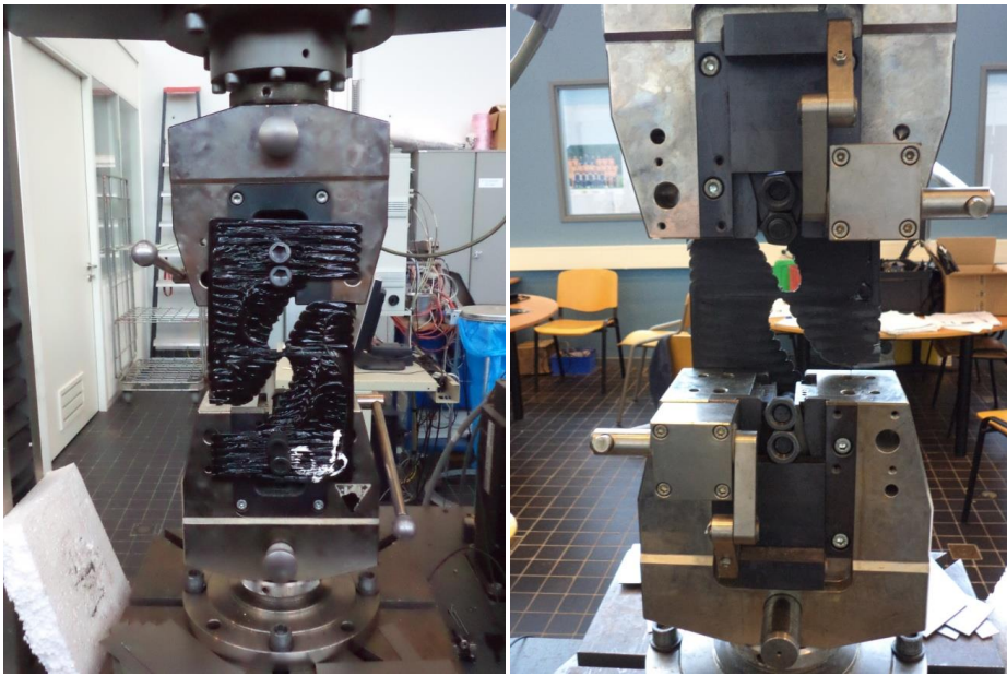
Fig. 55 Test setup for shear specimens that are printed within the xy-plane.
