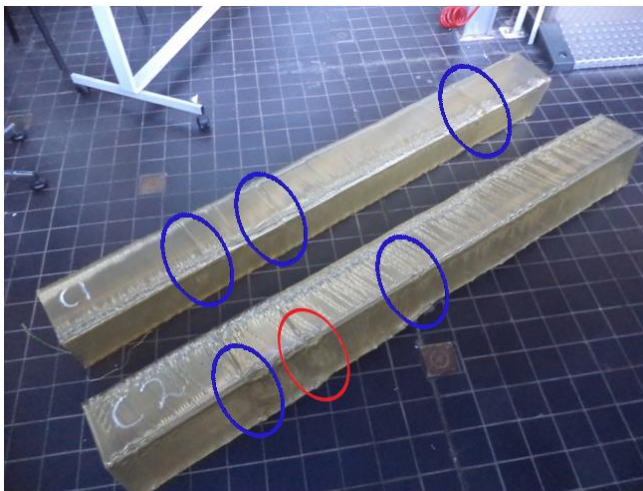
Fig. 145 Local inaccuracies that were observable on the C-geometries, prior to the test. The red-circled spot on geometry C2 is the location where rupture would take place during the test.
