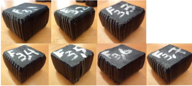
Fig. 69 Tested specimens that were loaded in direction 3
