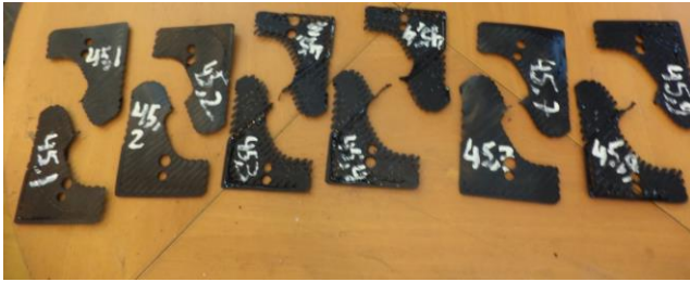
Fig. 60 Tested samples printed in the xy-plane and loaded in shear 45 degrees to the grain
