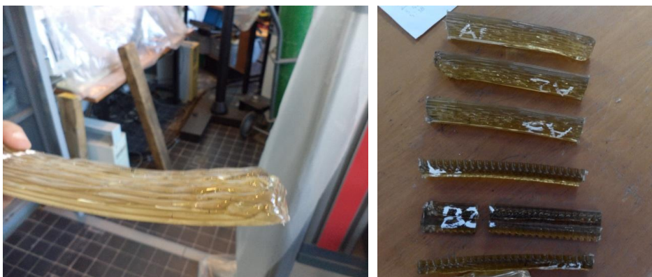
Fig. 133 Left: Permanent deformation of Block type A (left) and all the tested solid blocks (right)
