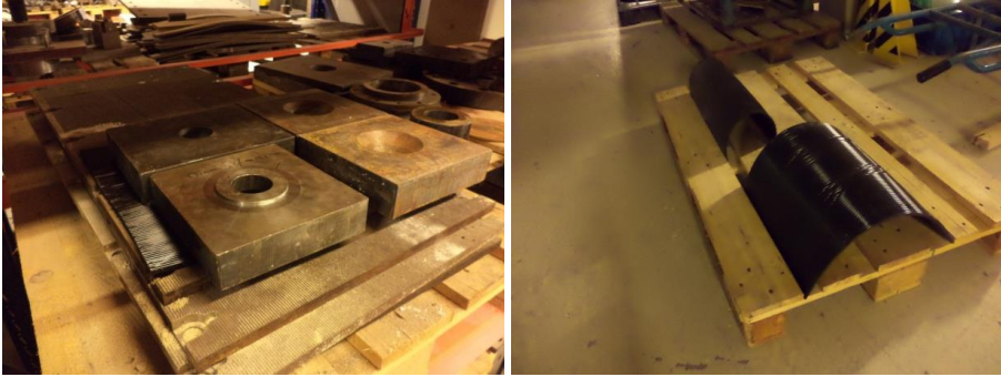
Fig. 34 Attempts to decrease the curvatures of the plates by placing weights on the plates and curving them in the opposite direction of the internal curve
