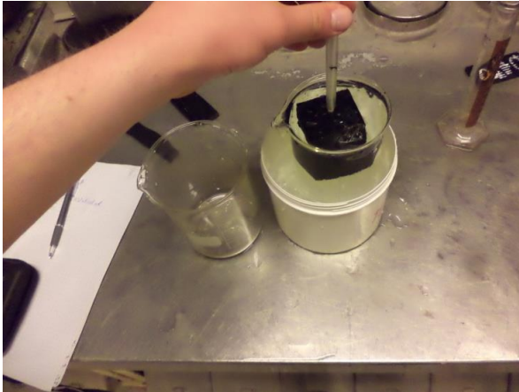
Fig. 77 By immersing the test sample and collecting the water that flows over the edge, the volume of the test specimen is determined
