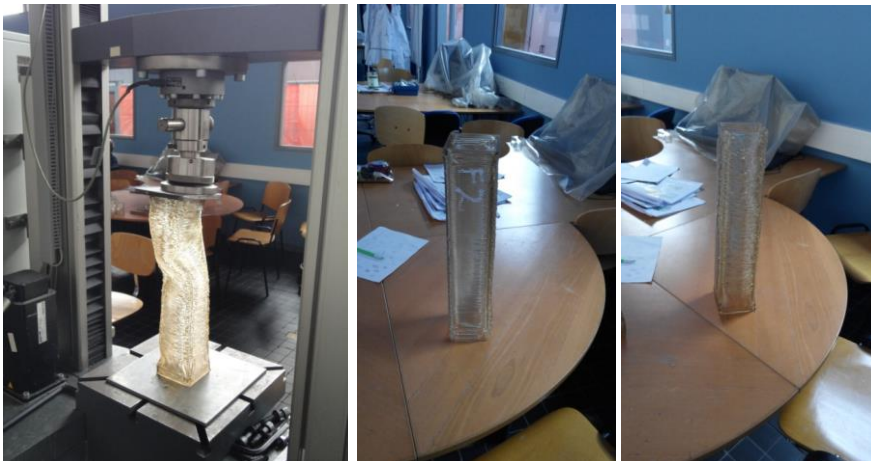
Fig. 117 Column F2 during and after the test. The sample seems to fold back completely.
