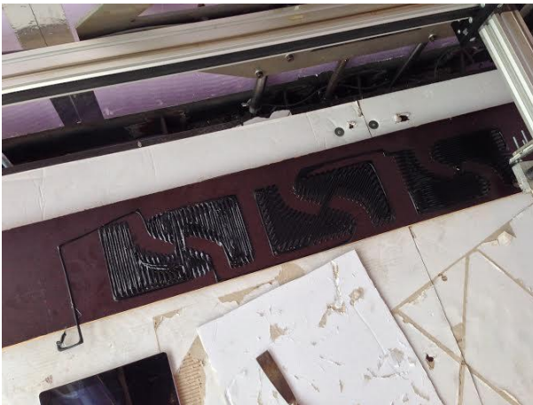
Fig. 27 Shear-specimens printed within the 'KamerMaker'
