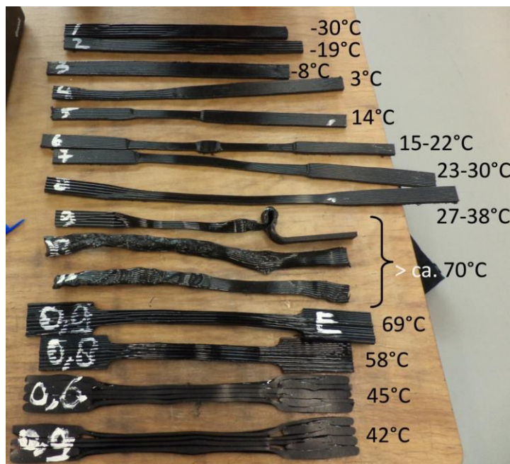
Fig. 83 Tested specimens and their surface-temperatures during the test
