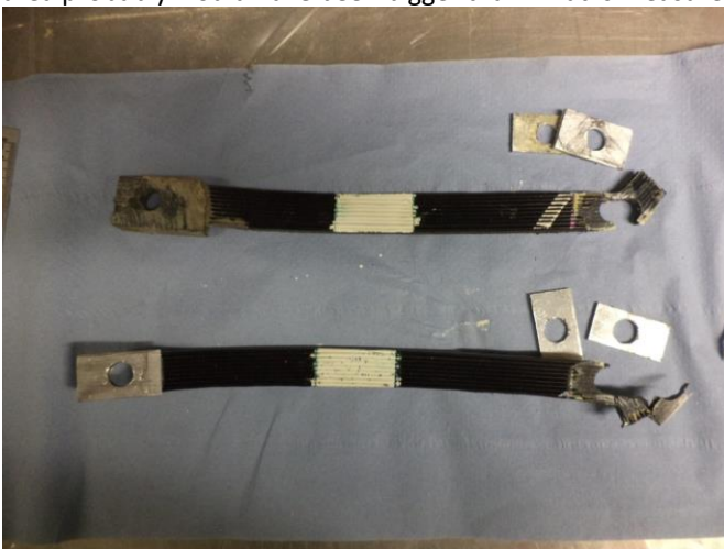
Fig. 95 Failed test specimens. As can be seen the specimens failed at the connection points
