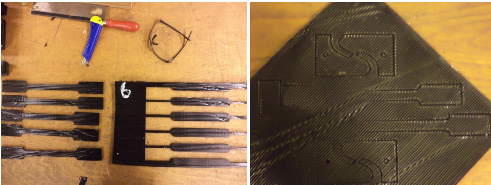
Fig. 35 Left: in case of straight plates, the samples are perfectly cut out from the plates. Right: In case of curved plates, the laser did not fully cut through the plate, such that using a fretsaw was required to obtain the sample.
