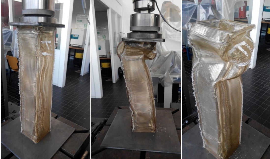
Fig. 116 Test-Column F1, during the test and directly after the test
