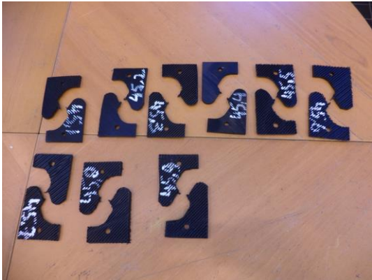
Fig. 53 Specimens printed within the xz-plane and loaded 45 degrees to the grain
