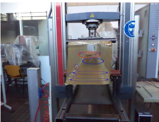
Fig. 146 Local inaccuracies in block C2, observable right after application of the load. As can be seen, the rupture process around the red-circled weak spot already starts right after the application of the load.
