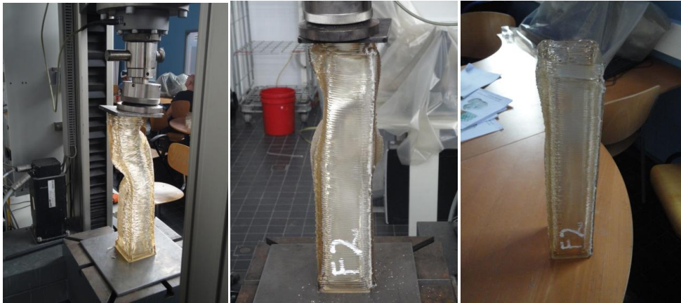
Fig. 118 Testing the column F2 for a second time. This time a small permanent deformation at the side is visible after the test (picture right).
