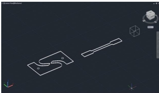
Fig. 24 3D-cad designs of the test specimens
