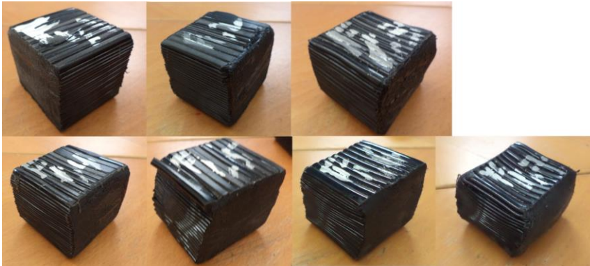
Fig. 65 Test specimens that are loaded in direction 1
