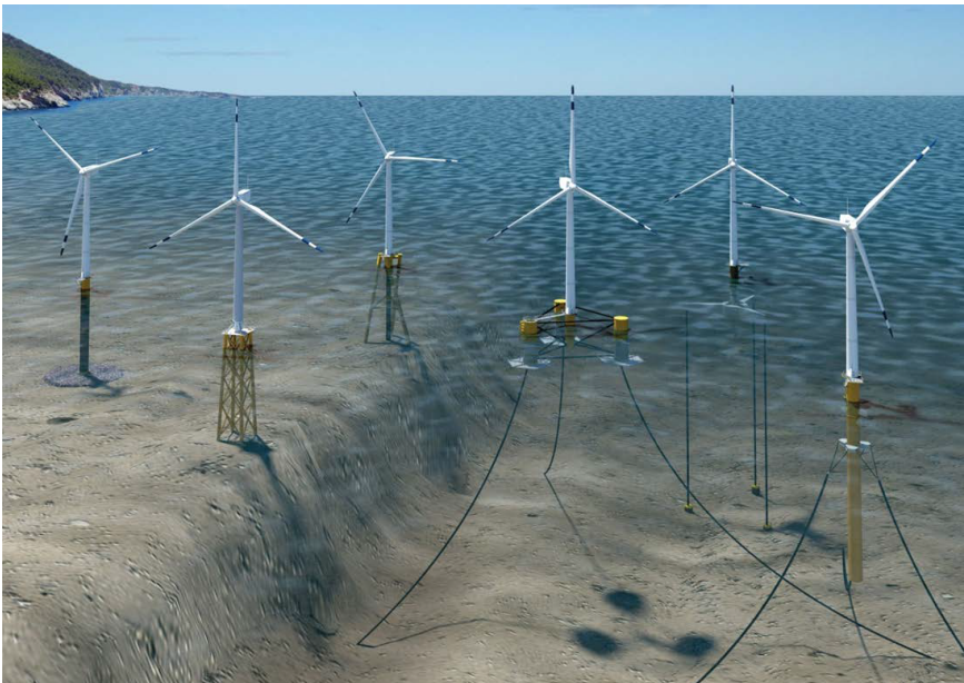
Figure 1.1: Various concepts of offshore wind substructures based on water depth - after Smith et al. [23].
