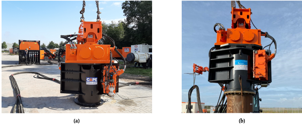
Figure 5.1: The GDP shaker: (a) view at the manufacturing site; (b) shaker connected to a test pile via a bolted flange connection
