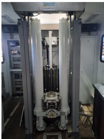
(a) Whole Setup Of Push frame, Automatic Placing Mechanism, Tube Storage And Raptor.
