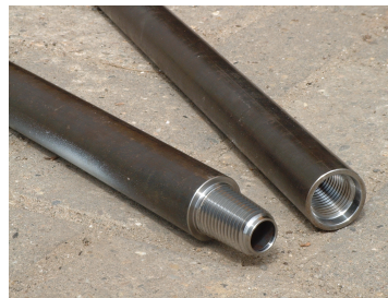
Figure 1.2: Ends Of CPT Tube To Mount Tubes On Top Of Each Other.
