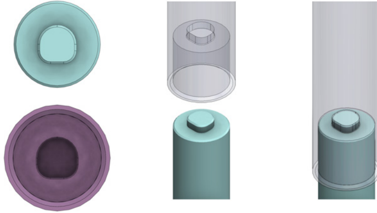
Figure 3.2: The end-effector and pillar interface. The dedicated asymmetric plug and hole design enables 6-DoF constraints of the entire SUTA kinematic configuration. Top left shows the pillar, bottom left the end-effector profile. The middle and right images illustrate the end-effector fitting over an artefact pillar.
