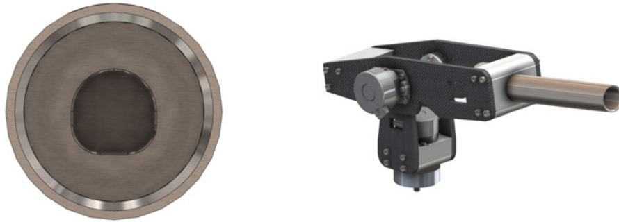
Figure E.2: Front- and isometric CAD view of the final steel end-effector with debossed interface profile used for all results in Chapter 4.
