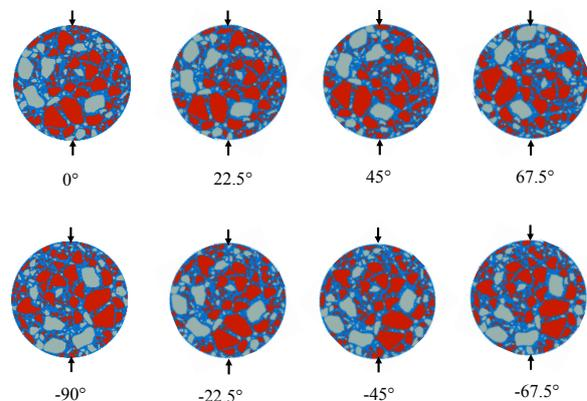
**Figure 9:** Different loading orientations on the image.
