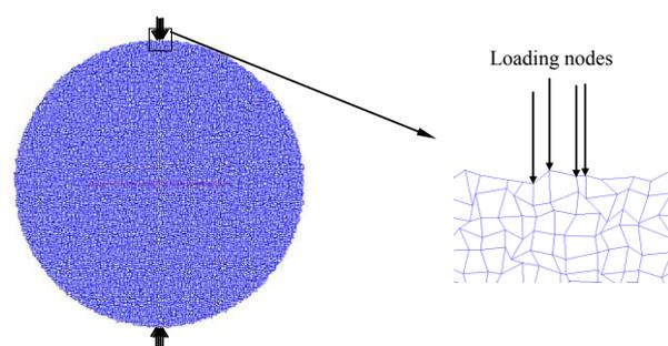
Figure 6 Illustration of simulation loading on the specimen.
