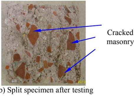
**Figure 2:** Set-up for indirect tensile test (a) and split specimen after testing (b).
