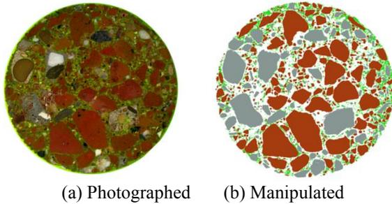
**Figure 3:** Image of a diametrical cross section of CTM<sub>i</sub>G<sub>r</sub> used in the monotonic ITT (red: RMA; gray: RCA; white: matrix or mortar; green: void filled by resin).
