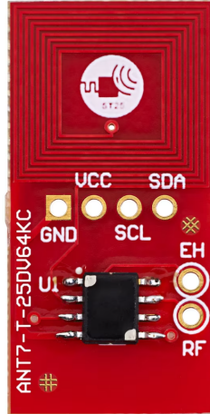
Figure 3.4: Top view of the ANT7-T-25DV64KC 14 mm \times 14 mm double layer antenna reference board
