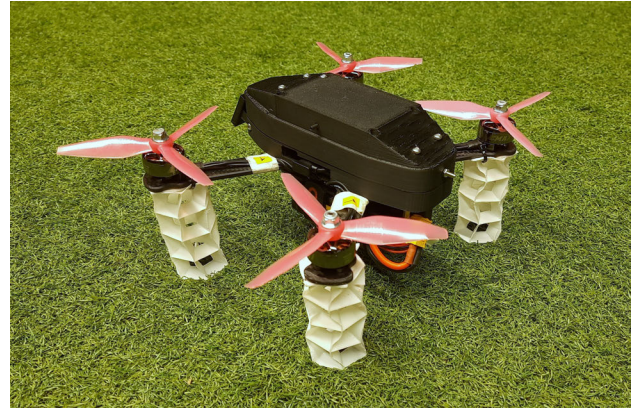
Fig. 1. A continuum twisted tower origami landing gear made of 4-stack hexahedric units mounted on a drone.
