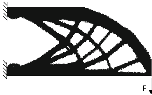
Figure 5.6: The topology optimization results of the example in Figure 15 in Rozvany et al. [1995], as generated by Beghini et al. [2014]
