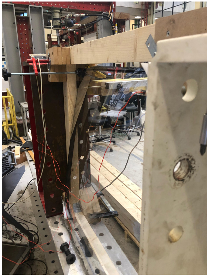
Figure 94. The maximum bend deflection (own work)
