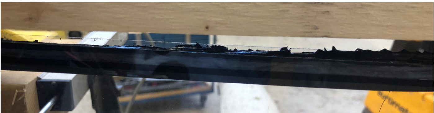
Figure 96. Secondary adhesive letting loose (own work)
