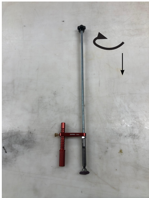
Figure 52. Configuration of the pushing screw (picture taken by author)
