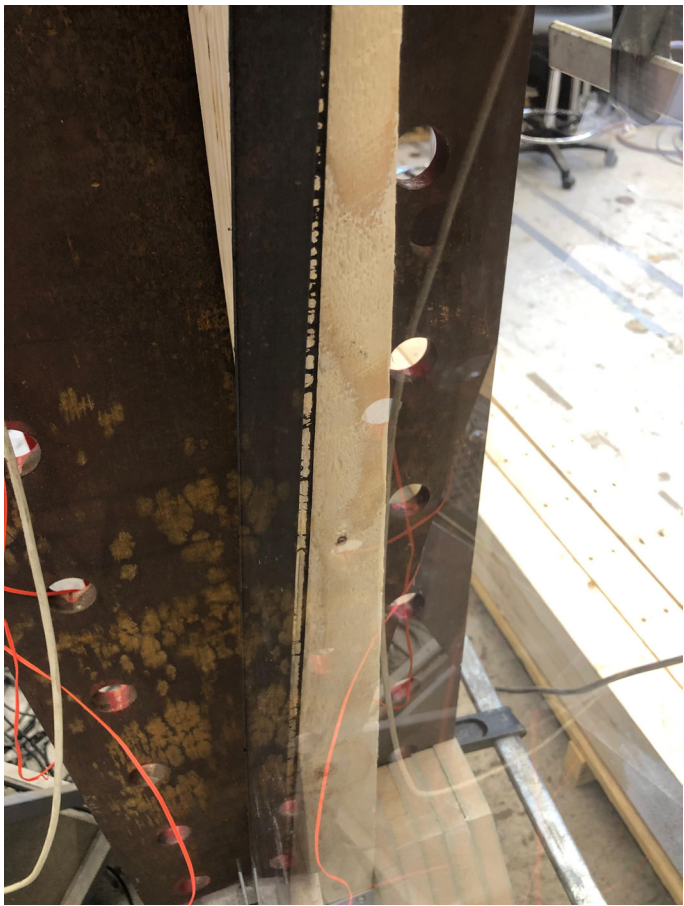
Figure 95. Polyisobutylene layer letting loose from the PMMA pane. (Own work)
