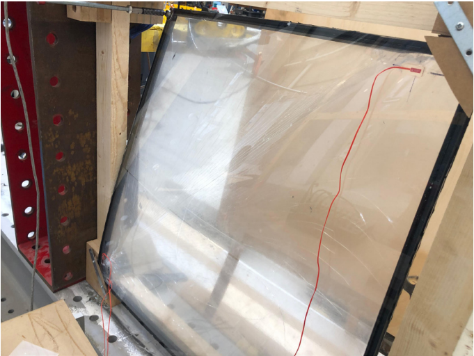
Figure 101. Panel after breakage of the back panel (Picture taken by author)
