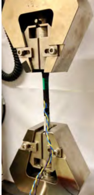
Figure 33. Set-up of the tensile dumbbell test. (fedoseeva, 2017)
