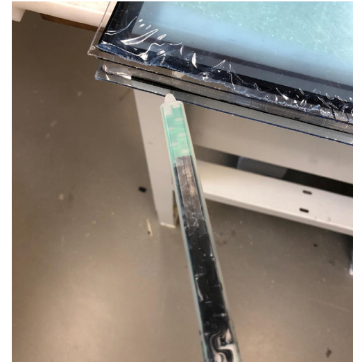
Figure 47. Application of the Ködiglaze S (Picture taken by author)
