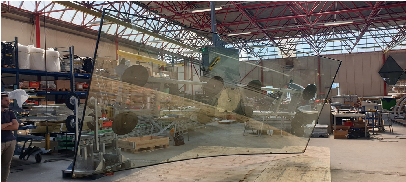
Figure 130. Cold bending mechanical system (Octatube, 2021)
