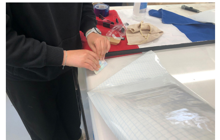
Figure 49. Lamination of one of the two laminated IGU's. Bookcover foil was used for its adhesion and strength. On these IGU's one innerpane and another outer pane were laminated. (Picture taken by author)
