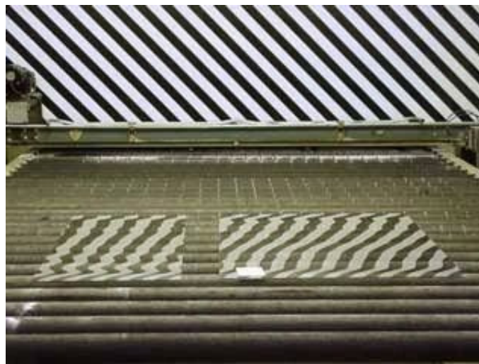
Figure 22. Roller wave distortion (Abbot, M. et al, 2001)
