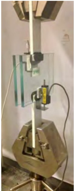
Figure 34. Set-up of the double-lap shear test. (fedoseeva, 2017)
