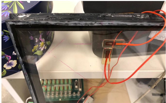
Figure 89. Double strain gauge setup in the corner (Own work)
