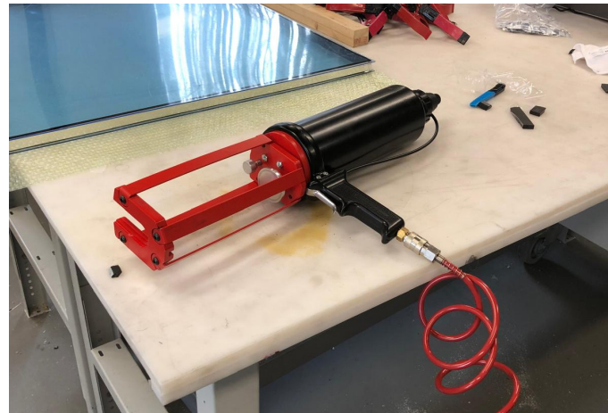
Figure 42. Innotech Rott Airflow one pneumatic dispenser (Picture taken by author)
