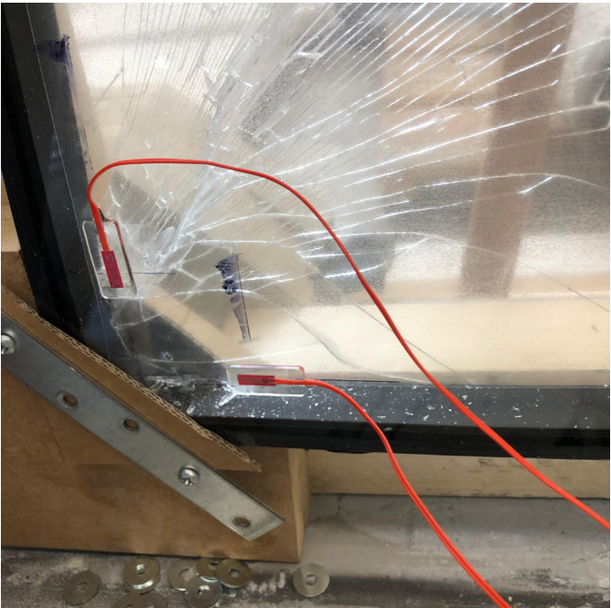
Figure 102. Panel at the clamp after breakage of the back panel (picture taken by author)
