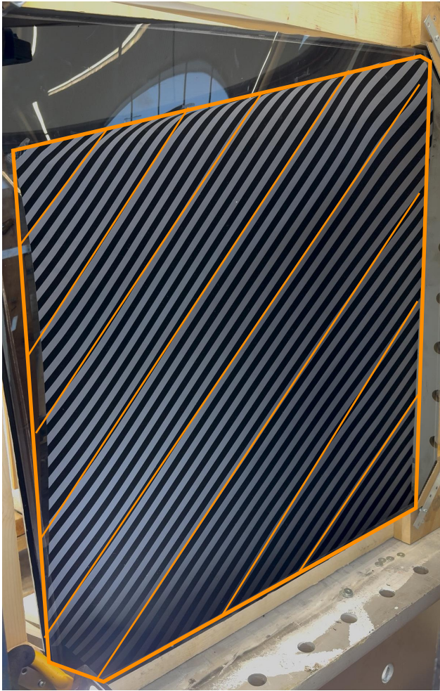
Figure 120. Zebra pattern after cold bending (Own work)
