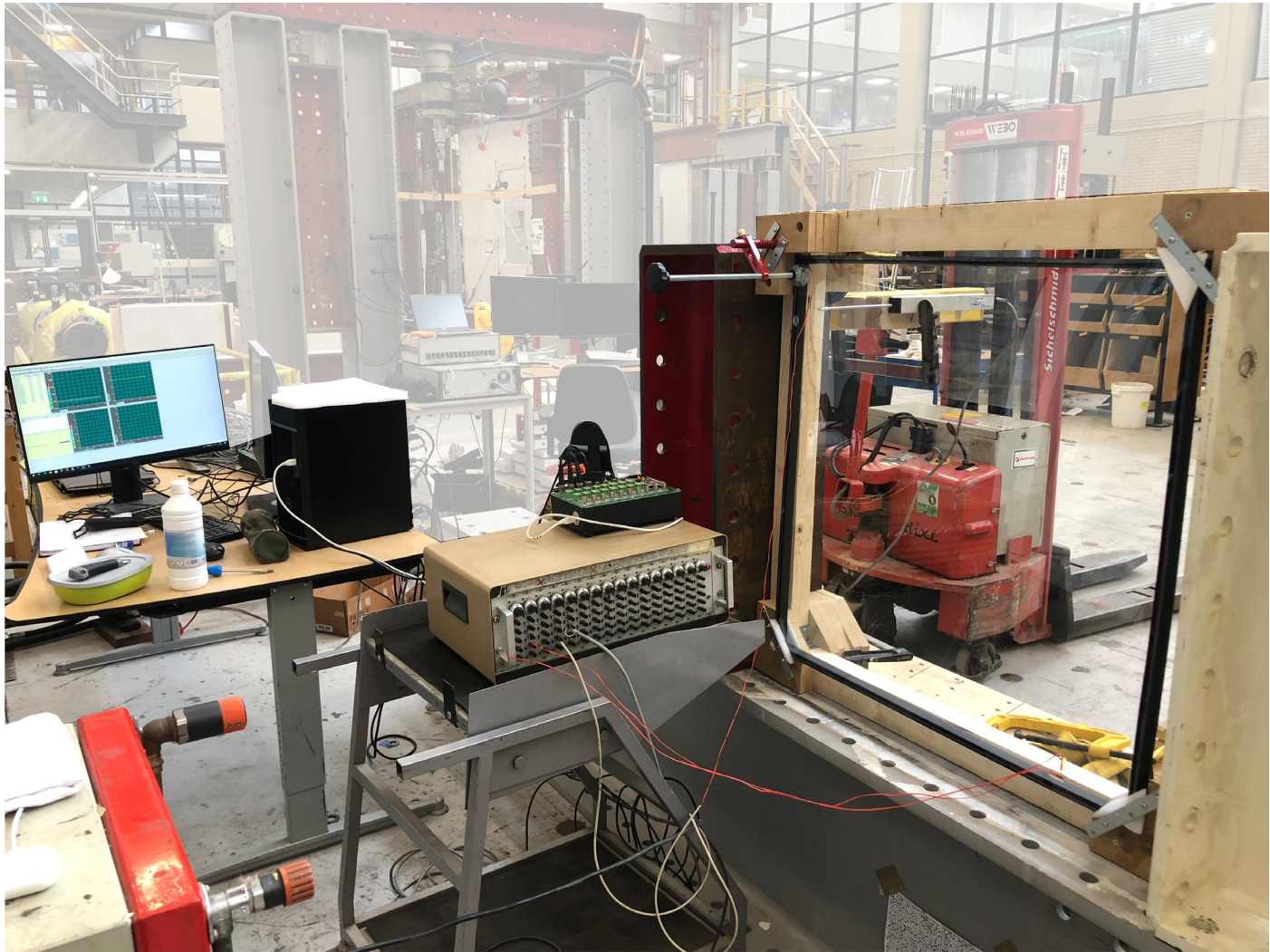
Figure 92. Complete single corner bending test setup.
