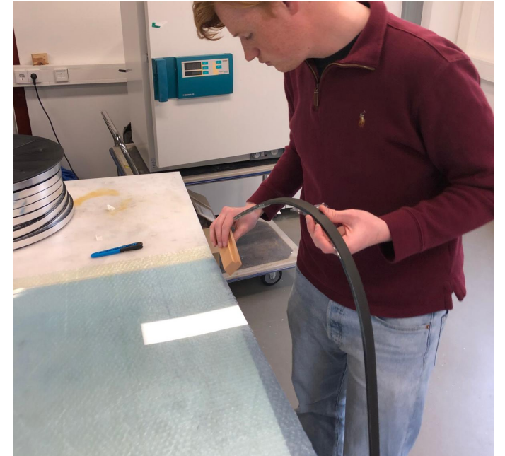
Figure 43. Application of the Triseal spacer (Picture taken by author)
