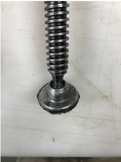
Figure 54. Tip of pushing screw, ball joint accommodates movement of the glass (picture taken by author)
