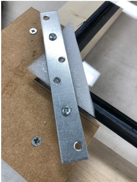
Figure 53. Clamped plexiglass panel (picture taken by author)
