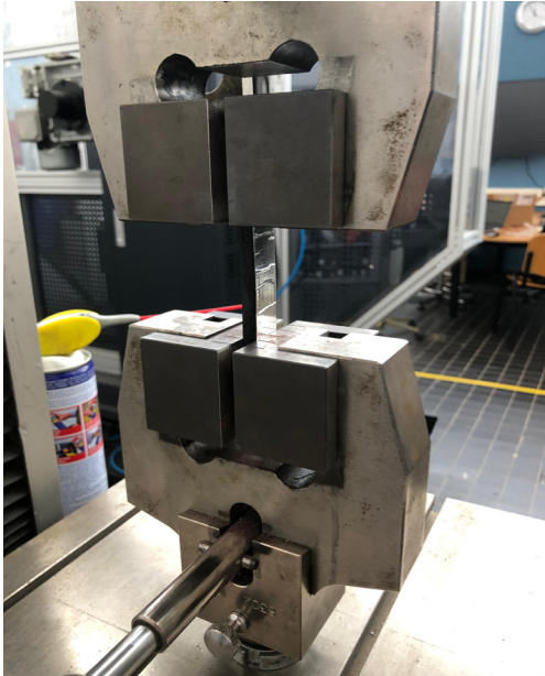
Figure 69. Tensile test setup: initial position (own work)
