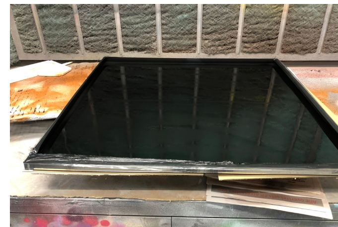
Figure 48. Black spray painted IGU, one inner pane is spray painted so that the reflection of the glass pane can be clearly observed (Picture taken by author)
