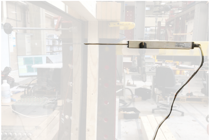
Figure 91. Displacement gauge setup behind the panel (Own work)
