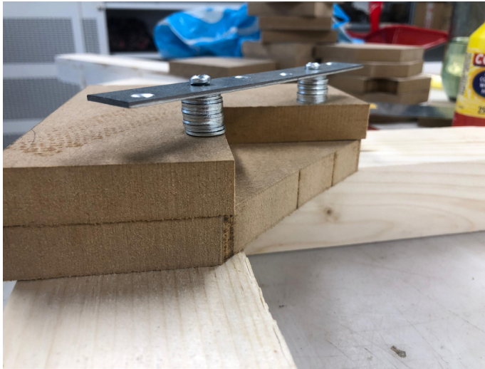
Figure 51. Final Design of the clamp (picture taken by author)
