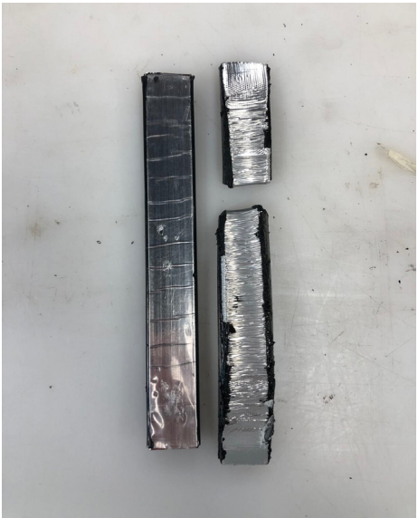
Figure 72. comparison of spacer before and after tensile test (own work)
