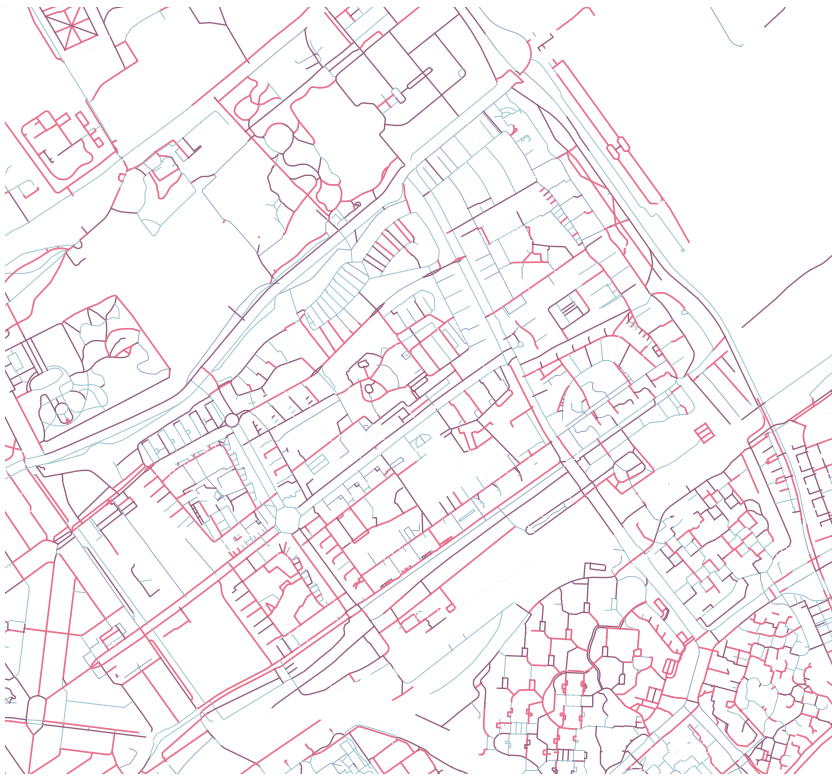
Figure 94 Local space syntax, with an integration distance of 800 metres
