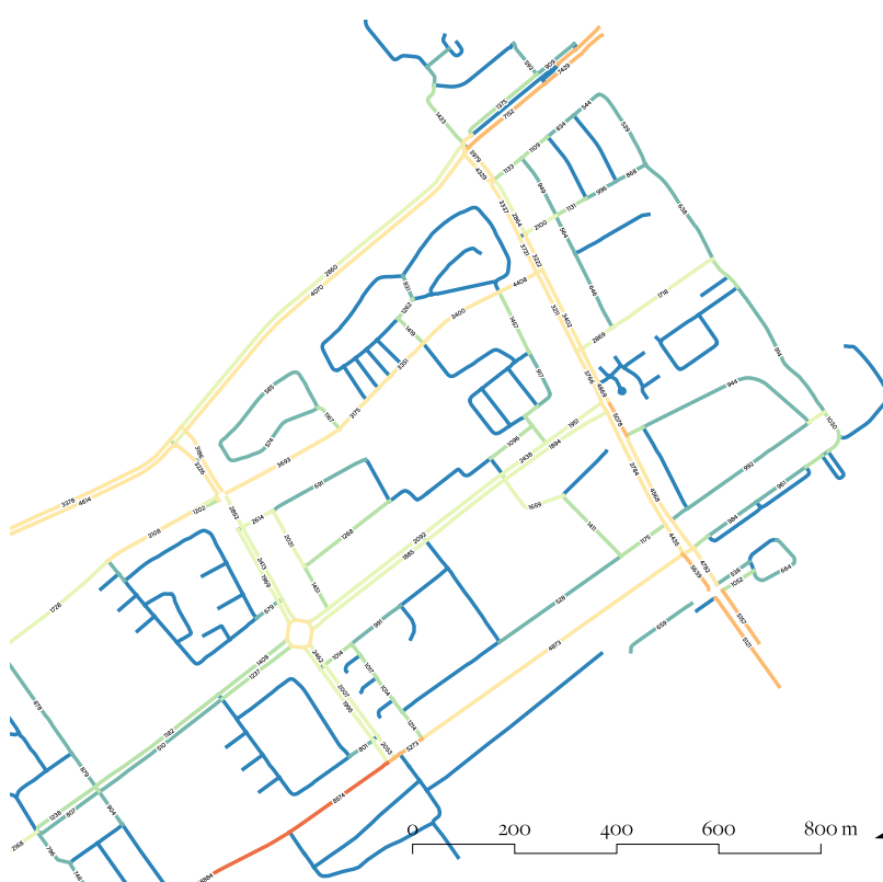
Figure 98 Average motor vehicle intensity map
