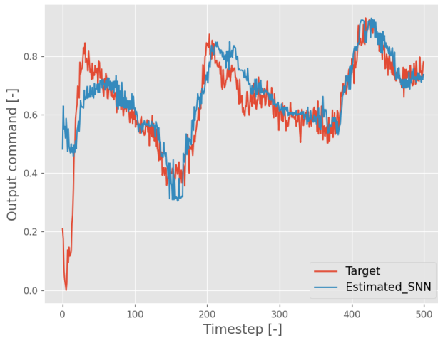
Fig. 13. The SNN controller estimations trained on a smoothed dataset generated with the reinforcement learning approach in comparison with target signal
