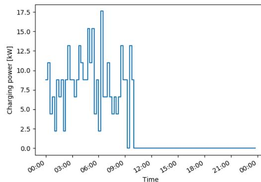
Figure 6.6: Optimised cumulative charging curve for a fleet of 9 EVs in *system design 16* including an ESS 01-01-2018
