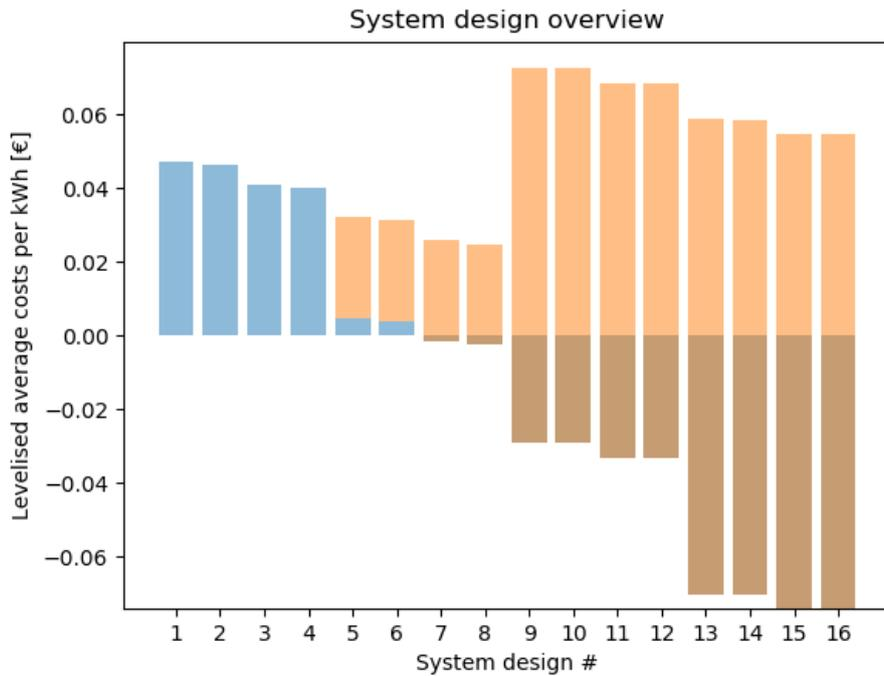
Figure 6.16: Grid capacity constraint 10% increase - system design performance
