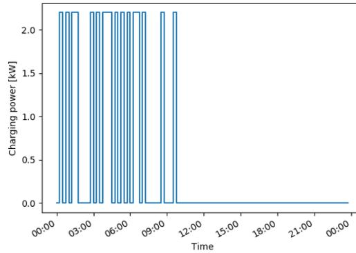
Figure 6.4: Optimised charging curve for a Single EV 01-01-2018
