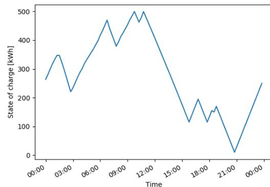
Figure 6.10: The state of charge of energy storage system 01-01-2018
