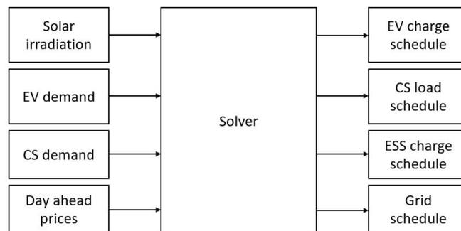
Figure 4.2: Schematic representation of the solver
