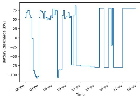
Figure 6.9: The (dis)charge of the energy storage system 01-01-2018
