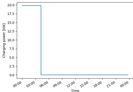
Figure 6.5: Conventional cumulative charging curve for a fleet of 9 EVs 01-01-2018
