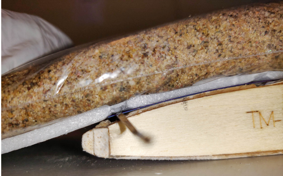
Figure 4.4: Application of the PV panel using the sand method
