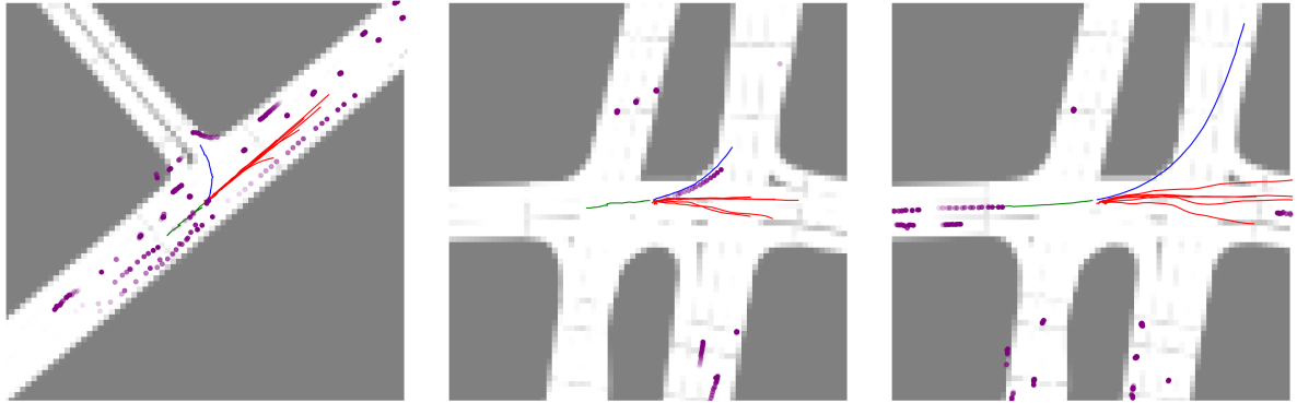
Figure 6.6: Examples of failed predictions, when the high-level goal is not predicted correctly. None of the predicted trajectories is correct, because the high-level network failed to predict the correct destination grid cell. The green line is an observed trajectory, blue is ground-truth trajectory, reds are the best 6 predictions. The purple dots are other vehicles, where the lightest purple are vehicles in the first timestamp and the darkest in the last observed timestamp.
