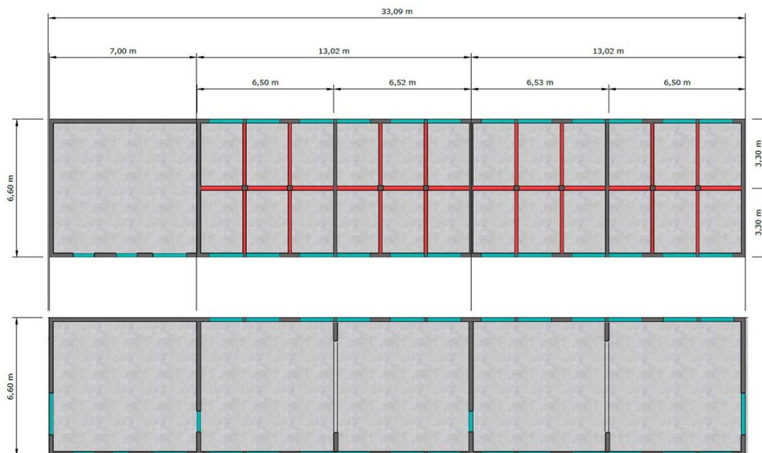
Figure 8.3: Concrete building floor plans
