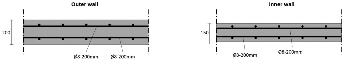
Figure 8.5: Concrete cross-sections: Outer walls (left), Inner walls (right). Units in mm
