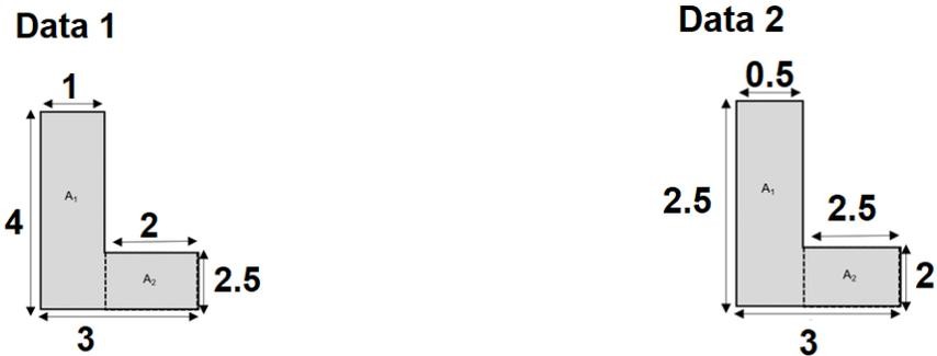
Figure H.3: Two different crown wall geometries
