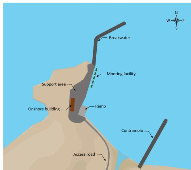
Figure 5.11: The final orientations of the main breakwater and contramolo
