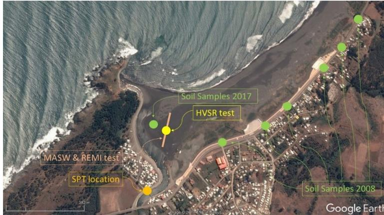
Figure 4.5: Map indicating the positions of the different tests performed (Google-Earth 2017).
