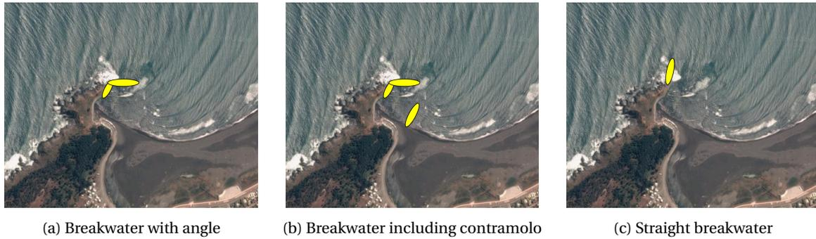
Figure E.4: Three configurations of the breakwater
