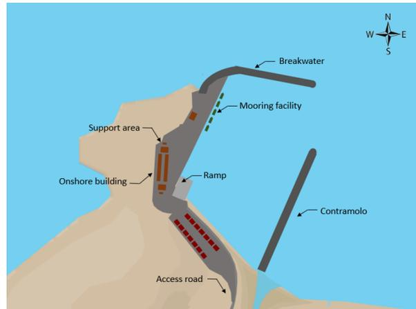
Figure 2.1: Schematic overview design proposal by the Department of Ports.
