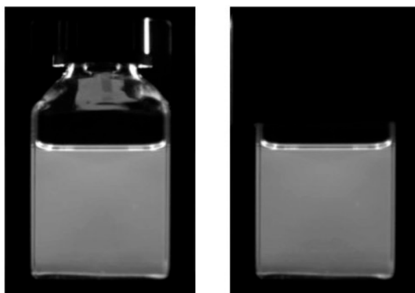
Figure 14. Images of the cell containing the fluorescent DPA solution. Left; no cover. Right; black paper cover over cap and shoulder of the cell.
