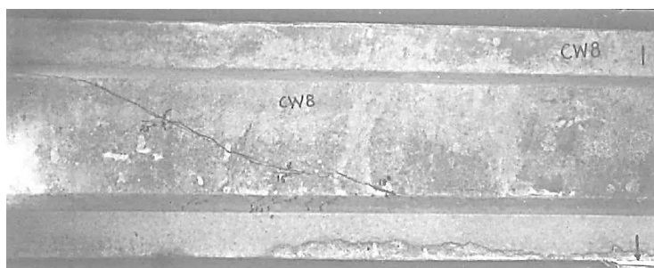
Figure 2.12. Photo at diagonal tension cracking of experiment CW8 (Elzanaty et al. 1986).
