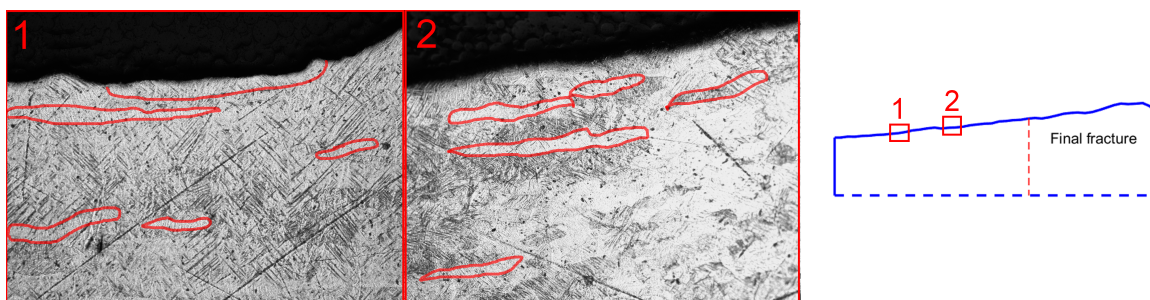
Figure 5.8: Crack path (90_4) - Prior beta grain in red
