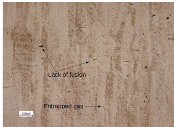
Figure 2.3: Initial defects present in SLM Ti-6Al-4V [3]
