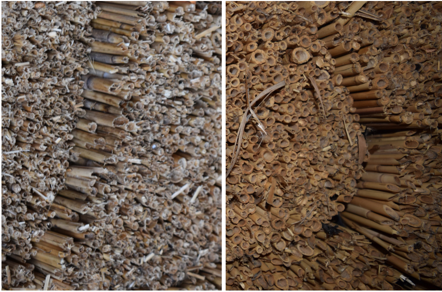
Figure 8: Reeds vary considerably in length, culm diameter and material properties. These images show Dutch reed (left) and Turkish reed (right). (By Author, 2019)
