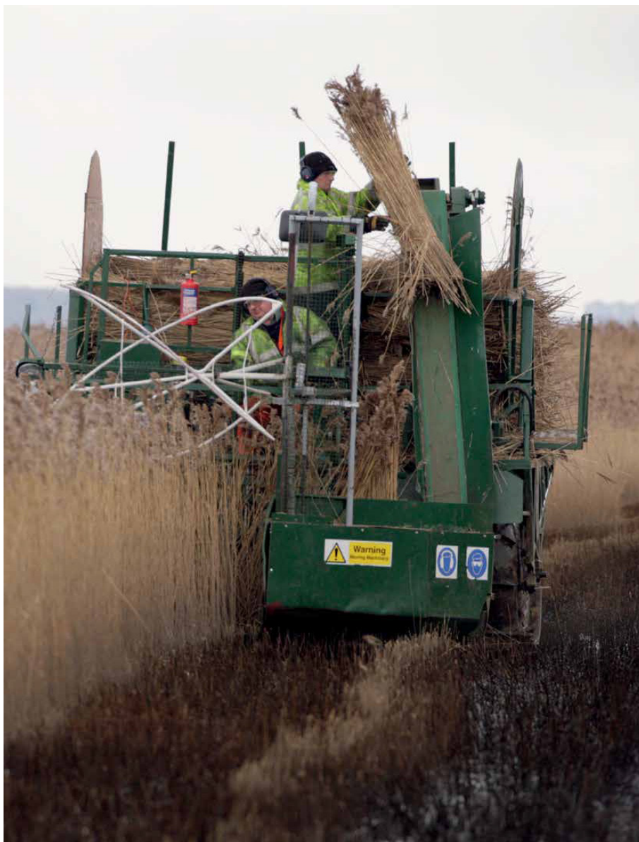
Figure 6: The Seiga Harvester is capable of cutting and tying around 1500 bundles of reed daily. Photo Credit: Andy Hay (White, 2014).
