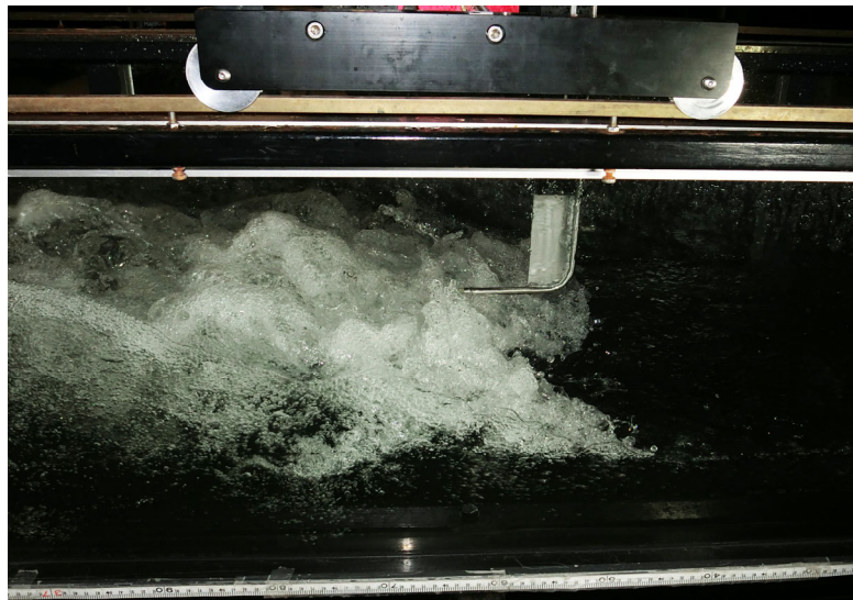
(B) Hydraulic jump for Fr_1 = 2.1 , Re = 1.97 \times 10^5 m, d_1 = 0.097 m, x_1 = 1.5 m, B = 0.5 m, shutter speed: 1/500 s - Flow direction from right to left, with the dual-tip phase-detection probe facing downstream
