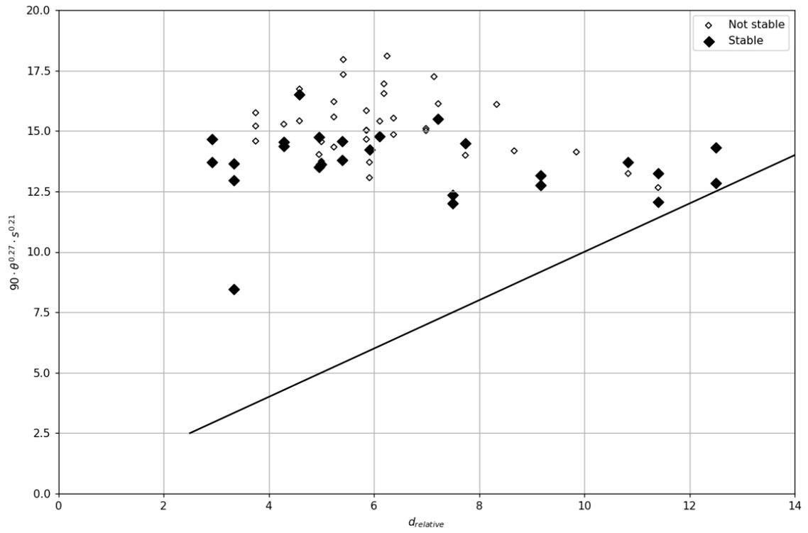
Figure E.5: Relation of the prediction method using the mobility parameter (from Section 4.4) with data points for the single plate (grey) reef using the spectral velocity determination
