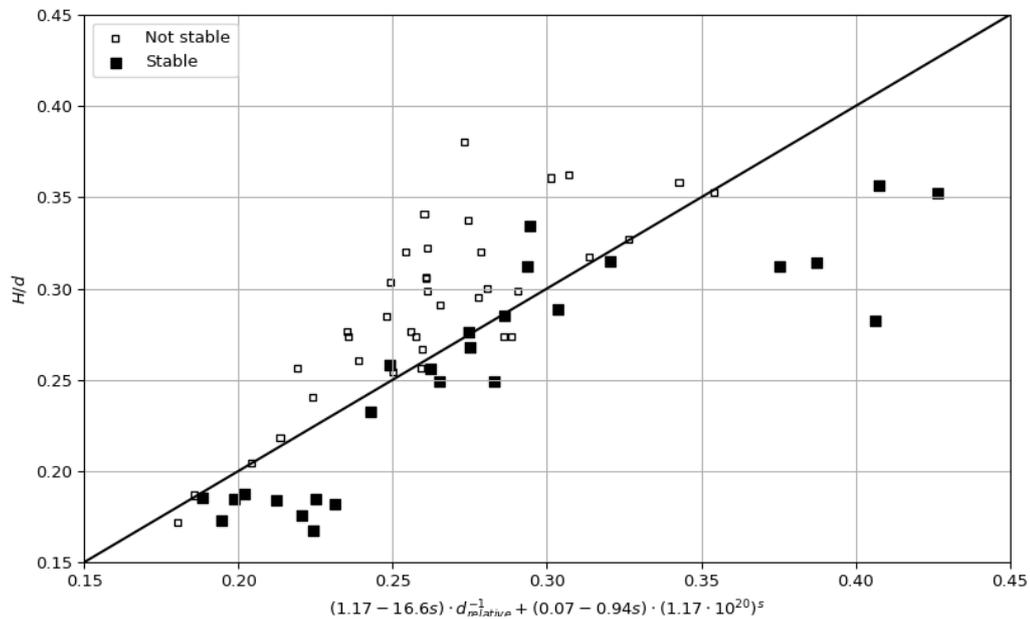
Figure 4.2: Relation of the resulting stability function for the single Stelcon plate (grey) reef with data points, with most of the unstable points above the line and stable points below
