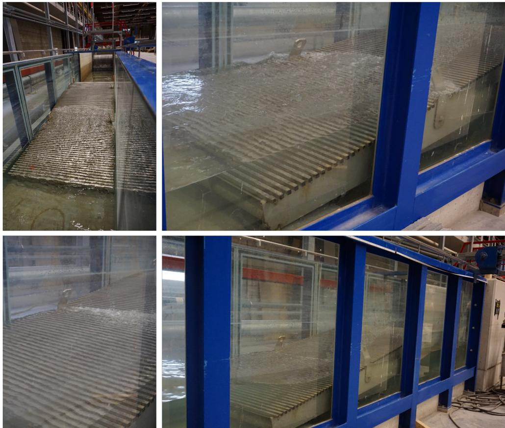
Figure 3.3: A wave absorber is positioned at the end of the flume to minimize reflected waves
