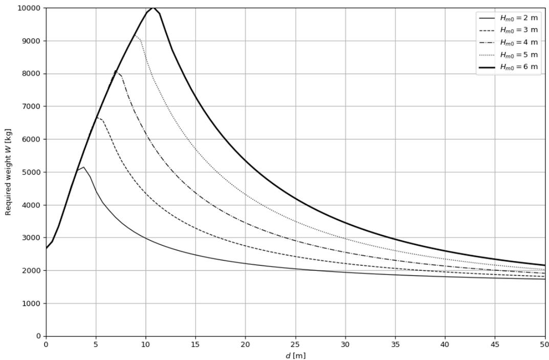
Figure 4.7: Relation between the required dry weight of the single plate reef prototype and the water depth for several significant wave heights according to the Morison stability prediction. A safety factor of 1.2 is used. The spectral period  $T_{m-1,0}$  is equal to 10 s.
