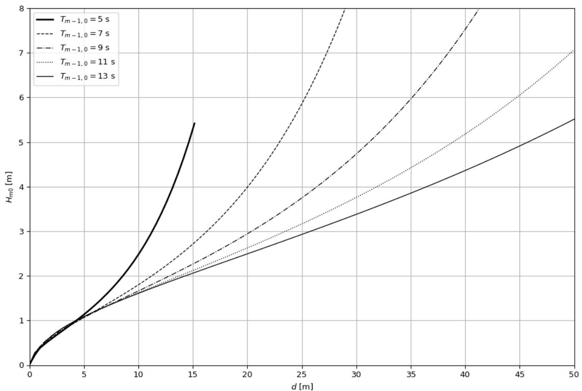
Figure 4.8: Relation between the significant wave height and the water depth for several spectral periods for the single plate reef prototype (2444 kg) according to the Morison stability prediction using a safety factor of 1.2. Above a curve, the reef is unstable, while below a curve the reef is stable.
