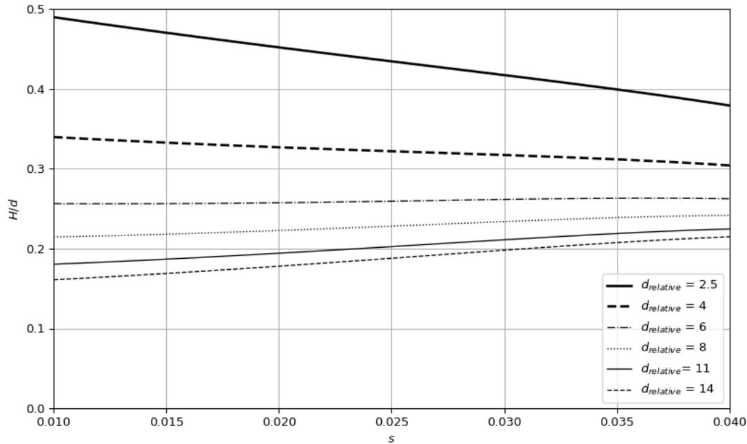
Figure 4.3: Plot for the resulting stability function for the single Stelcon plate (grey) reef
