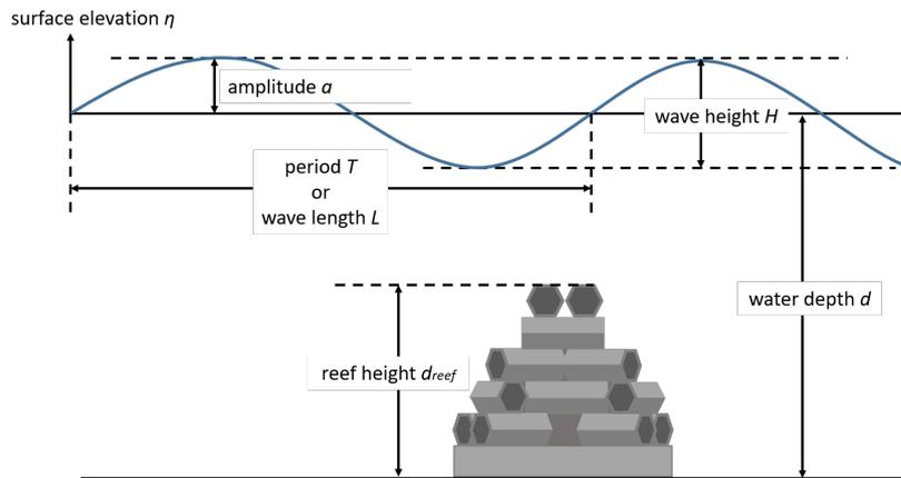
Figure 2.4: Overview of a propagating wave above a reef with reef height  $d_{reef}$
