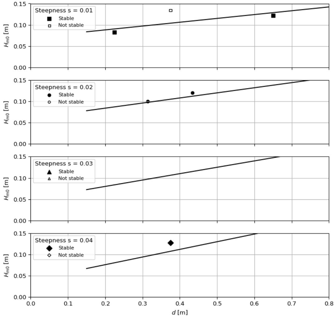
Figure G.1: Linear relation between the wave height  $H_{m0}$  and the water depth  $d$  for four different wave steepnesses. The plotted trend lines indicate the linear relationship, suggesting the extreme limit at which the reef just remains stable. The data points are obtained from the irregular wave tests for the pink reef model.
