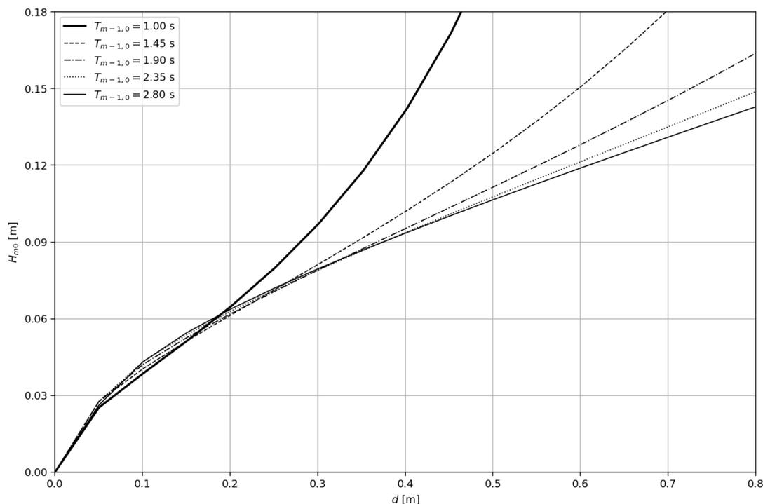
Figure 4.5: Relation between the significant wave height and the water depth for several spectral periods for the single plate (grey) reef model according to the Morison stability prediction
