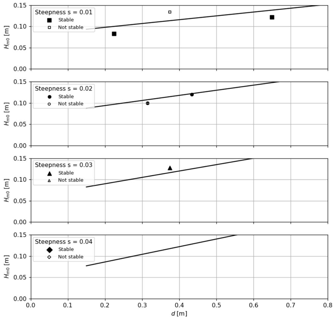
Figure G.6: Linear relation between the wave height  $H_{m0}$  and the water depth  $d$  for four different wave steepnesses. The plotted trend lines indicate the linear relationship, suggesting the extreme limit at which the reef just remains stable. The data points are obtained from the irregular wave tests for the 2x2 reef model.
