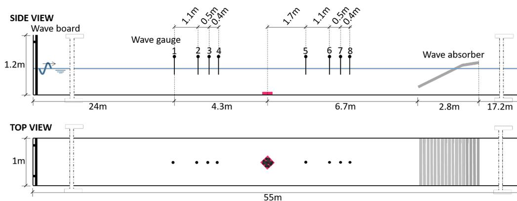
Figure 3.1: Experimental set-up of the flume
