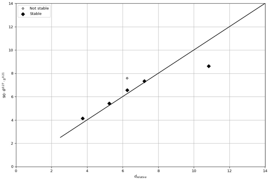
Figure G.9: Relation of the prediction method using the mobility parameter in which  $r_1 = 90$  for the 2x2 reef including data points
