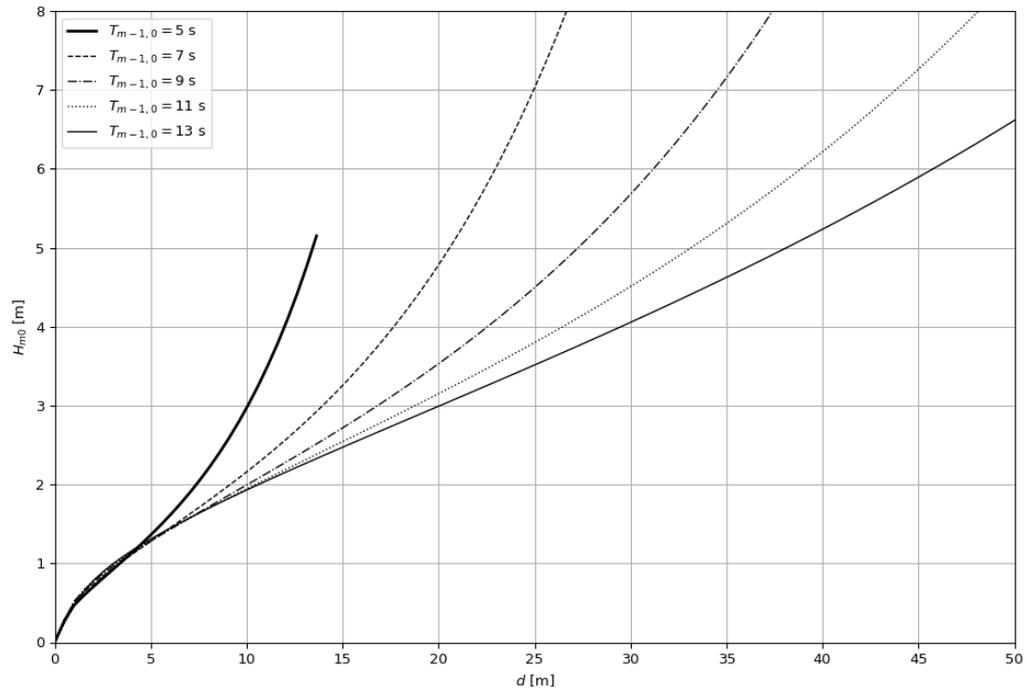
Figure F.2: Relation between the significant wave height and the water depth for several spectral periods for the single plate reef prototype according to the Morison stability prediction without a safety factor. Above a curve, the reef is unstable, while below a curve the reef is stable.
