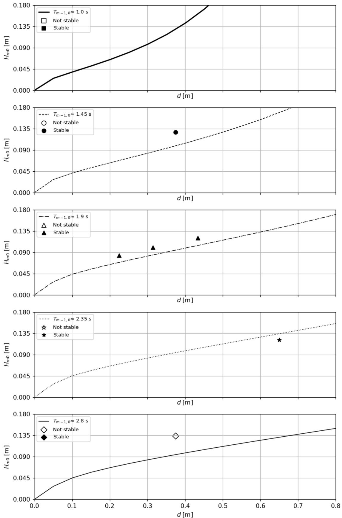
Figure G.8: Separate plots for the relation between the significant wave height and the water depth for several spectral periods for the 2x2 reef model according to the Morison stability prediction, including the data points of the flume tests
