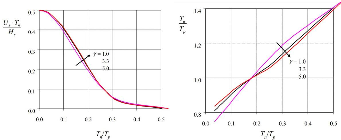
(a) By fitting a curve through some characteristic points on the graph for  $\gamma = 3.3$ , the relation between the x- and y-axis is determined and is as follows:  $y = 564.7x^6 - 857.3x^5 + 441.4x^4 - 73.92x^3 - 3.073x^2 - 0.2279x + 0.5009$ , in which  $x = T_n/T_p$  and  $y = U_s \cdot T_n/H_s$ .
