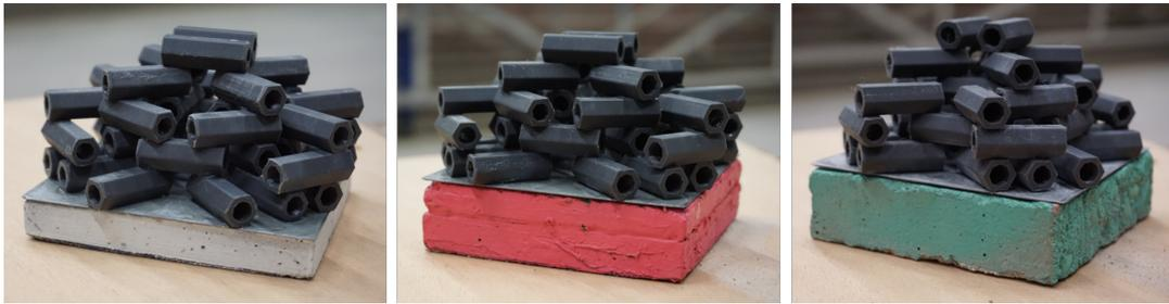
Figure 3.6: Models of the reefs, with a single (left), double (middle), or triple (right) layer of Stelcon concrete plates
