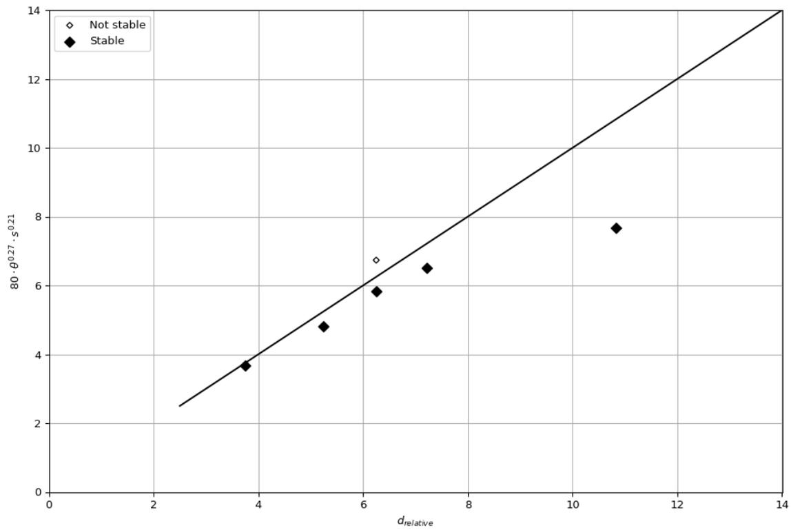
Figure G.10: Relation of the 2x2 reef specific prediction method using the mobility parameter in which  $r_1 = 80$  including data points
