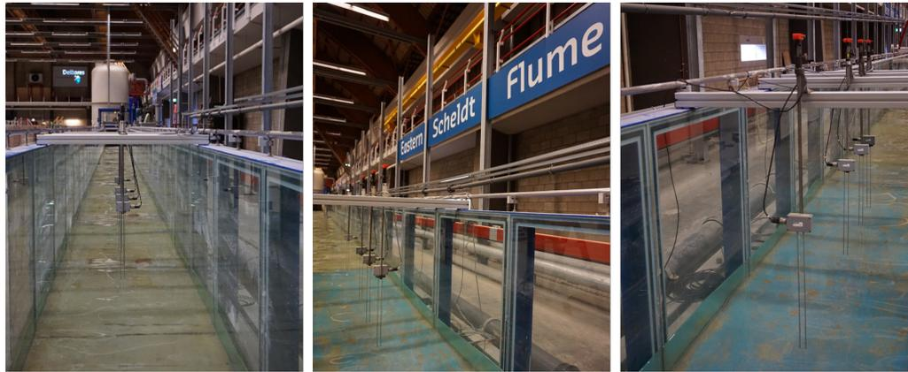
Figure 3.4: Impression of the wave gauges during the experiment
