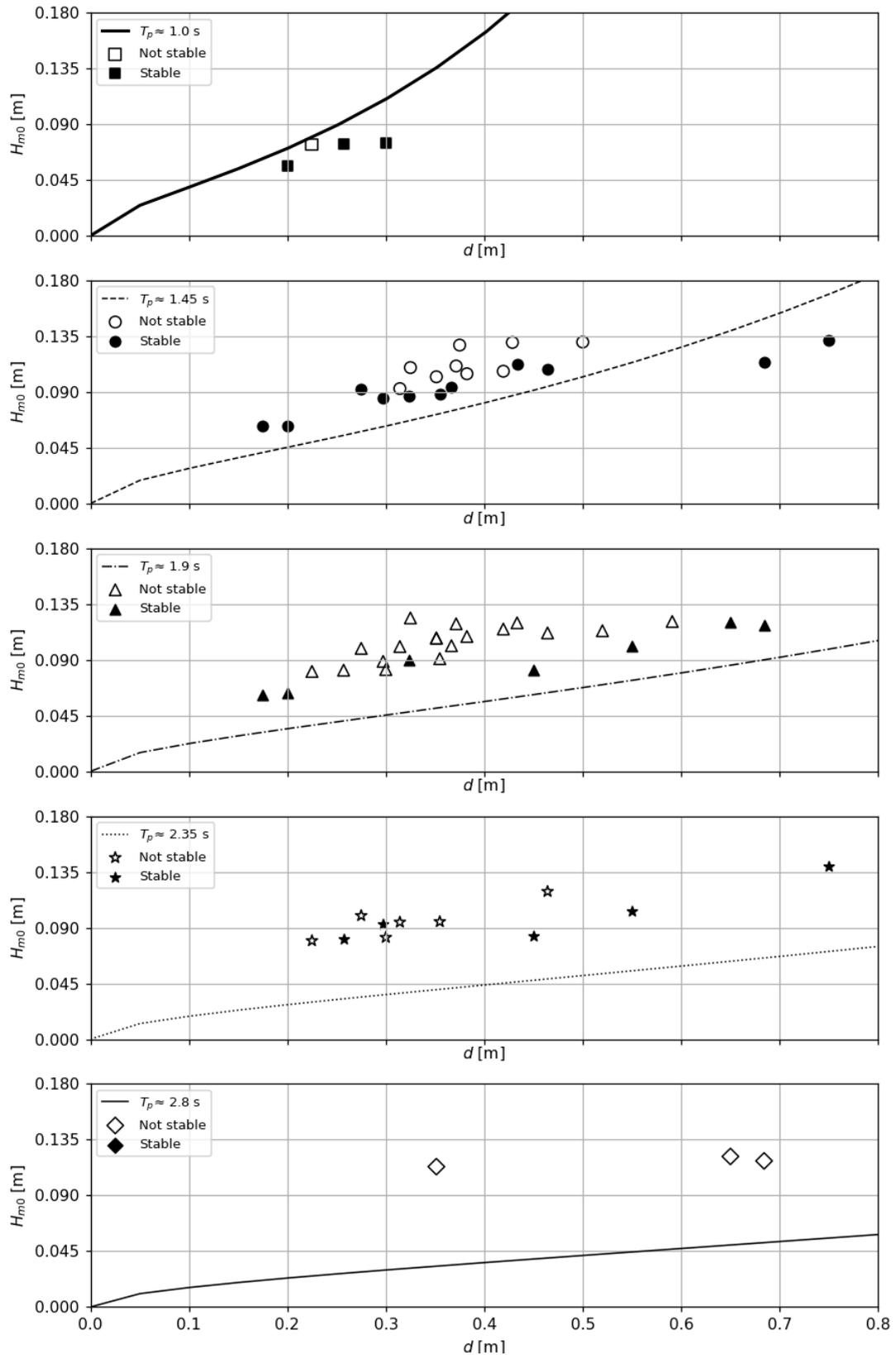
Figure E.3: Relation between the significant wave height and the water depth for several peak periods for the single plate (grey) reef model according to the Morison stability prediction using the spectral velocity
