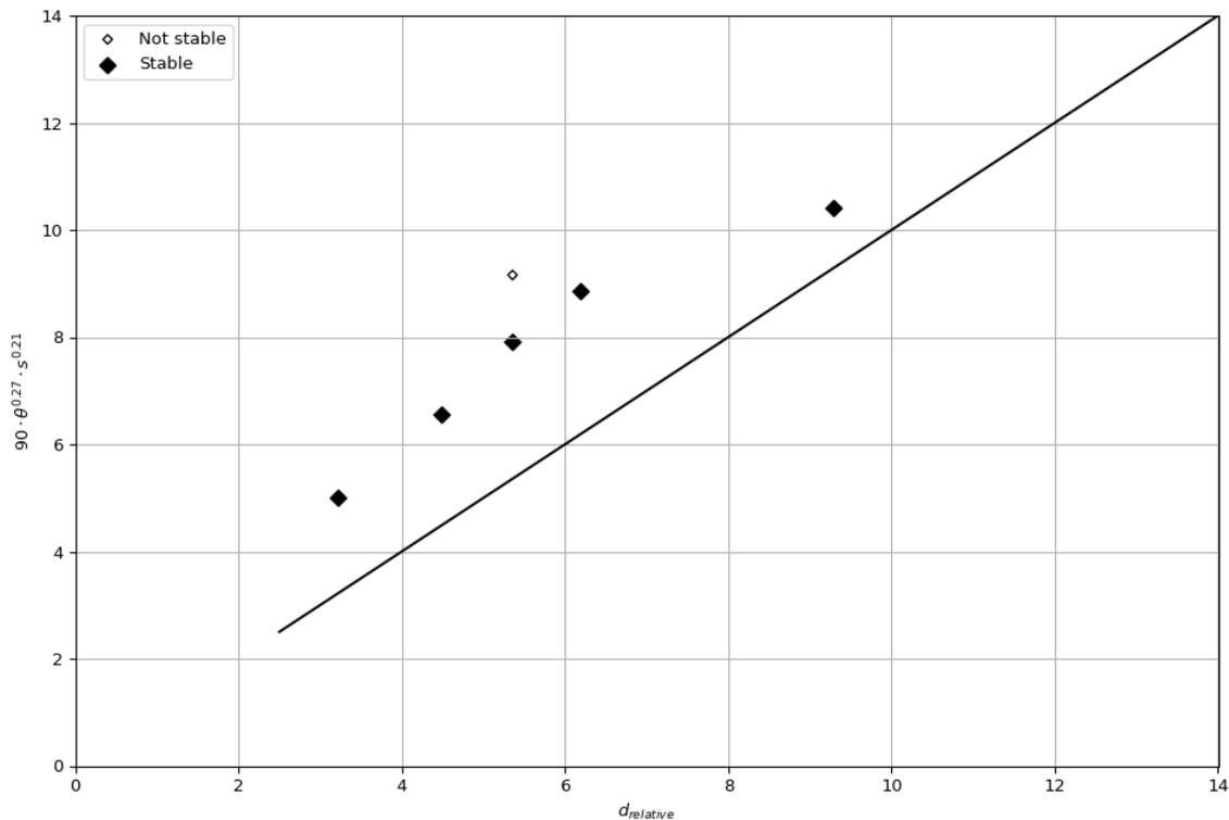
Figure G.4: Relation of the prediction method using the mobility parameter for the pink reef in which  $r_1 = 90$  including data points
