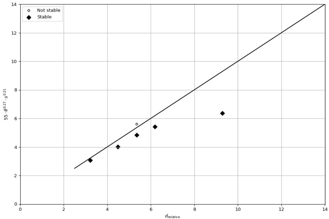
Figure G.5: Relation of the pink reef specific prediction method using the mobility parameter in which  $r_1 = 55$  including data points
