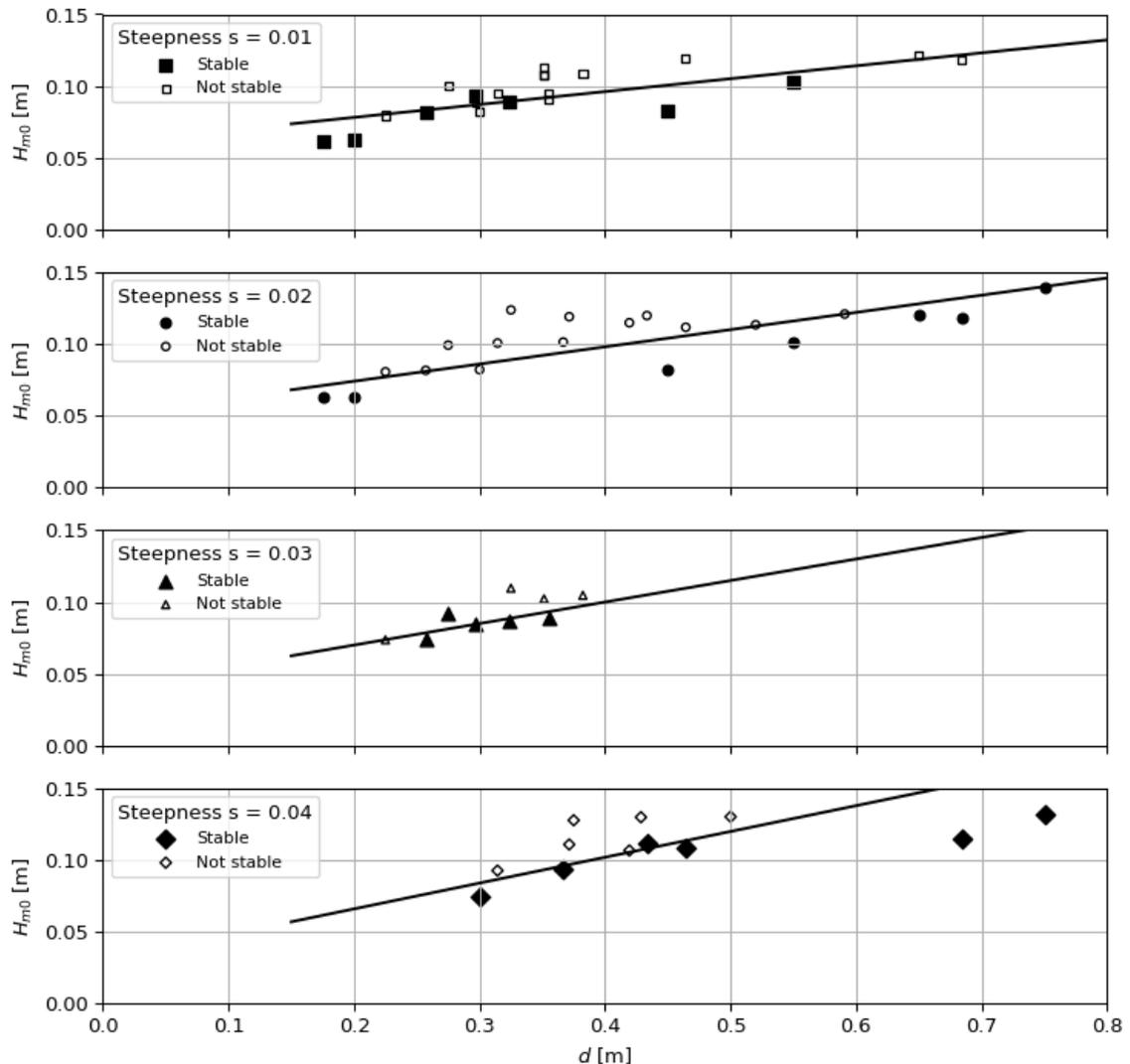
Figure 4.1: Linear relation between the wave height  $H_{m0}$  and the water depth  $d$  for four different wave steepnesses. The plotted trend lines indicate the linear relationship, suggesting the extreme limit at which the reef just remains stable, which is elaborated in Section 4.2.
