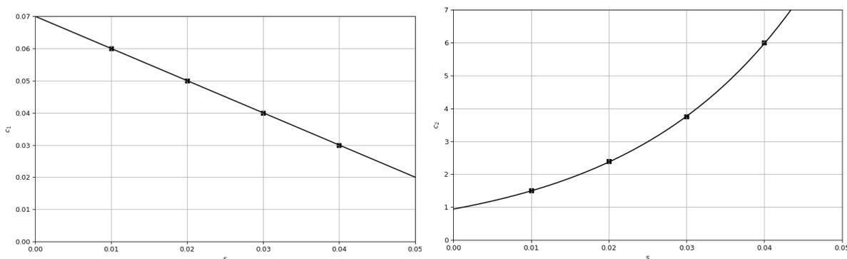
(a) The relation between the constant  $c_1$  and wave steepness  $s$ , which is equal to  $c_1 = 0.07 - s$
