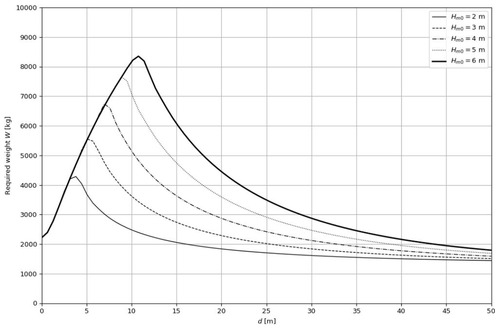
Figure F.1: Relation between the required dry weight of the single plate reef prototype and the water depth for several significant wave heights according to the Morison stability prediction without a safety factor. The spectral period  $T_{m-1,0}$  is equal to 10 s.
