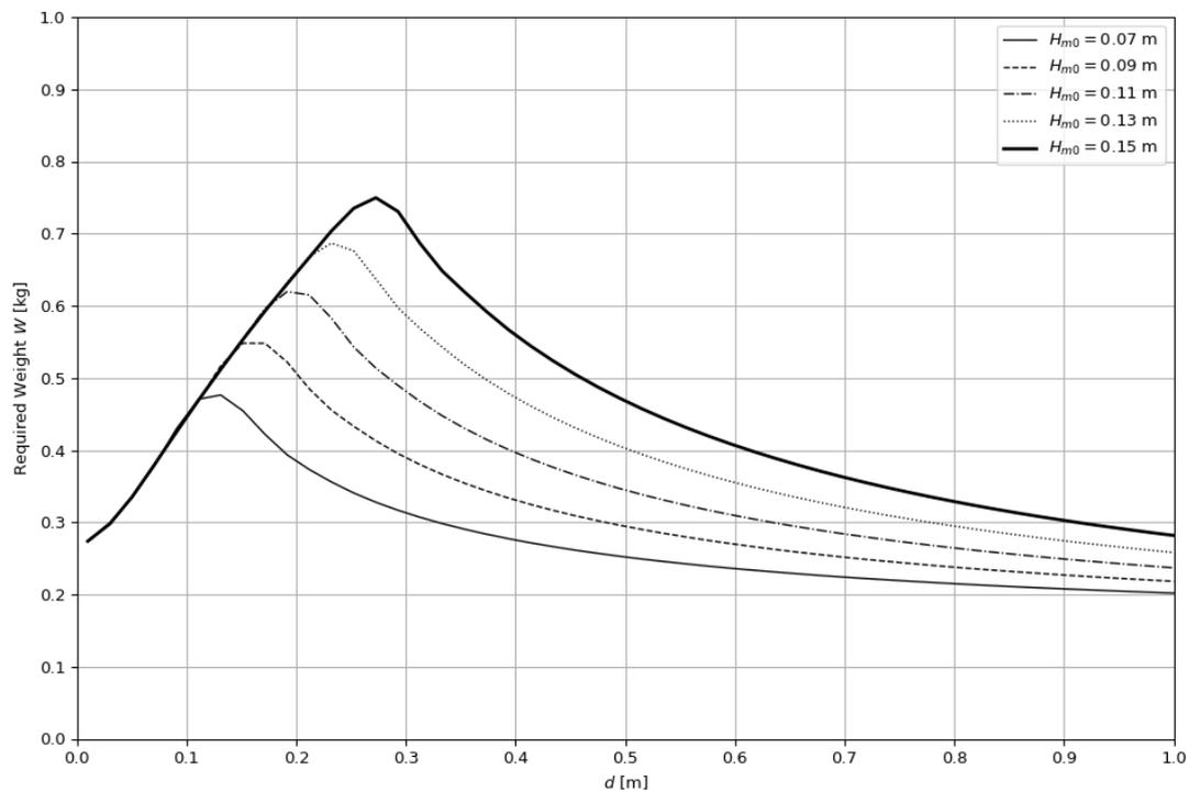
Figure 4.4: Relation between the required dry weight of the single plate (grey) reef model and the water depth for several significant wave heights according to the Morison stability prediction
