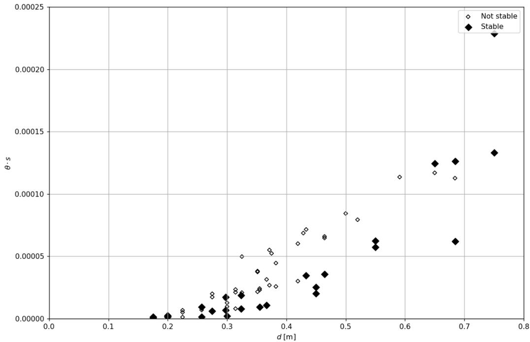
Figure 4.9: Data points from the experimental wave flume tests show the trend between the  $\theta s$ -value and the water depth  $d$  in meters
