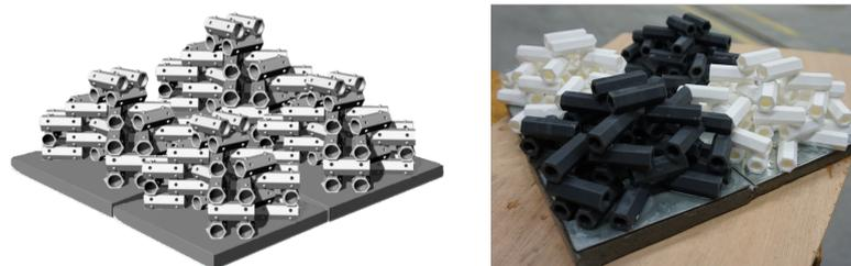
Figure 3.7: A schematic (left) and picture of the model (right) of the 2x2 reef. The deviation in color between the different reefs is due to the difference in printing material, but it has no further significance.
