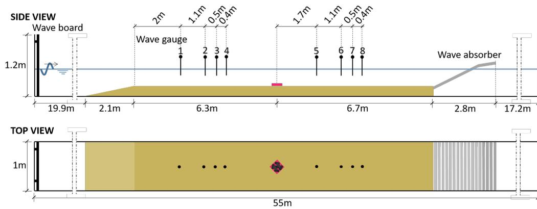
Figure 3.2: Experimental set-up of the flume including foreshore, which is installed after the fourth testing day. The foreshore is made of concrete and has a height of 20 cm
