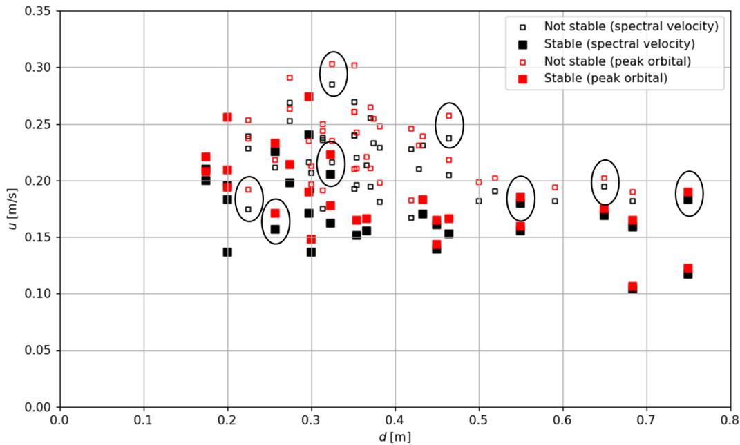
Figure E.2: Data points for which the velocity  $u$  is calculated with different methods; the black points are determined using the spectral velocity and the red points are determined using the peak orbital velocity as given in Equation 2.24, for which the significant wave height and spectral wave period,  $H_s$  and  $T_{m-1,0}$  are used.
