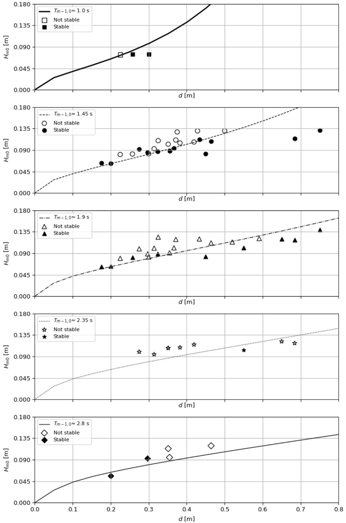
Figure 4.6: Separate plots for the relation between the significant wave height and the water depth for several spectral periods for the single plate (grey) reef model according to the Morison stability prediction, including the data points of the flume tests
