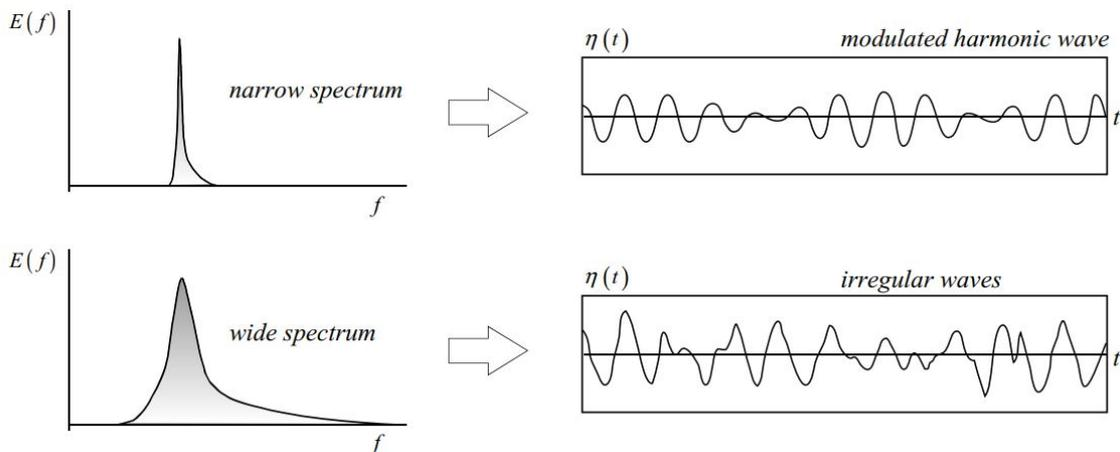
Figure 2.3: A narrow and a wide spectrum for swell waves and wind sea respectively with corresponding time series (Holthuijsen, 2007)
