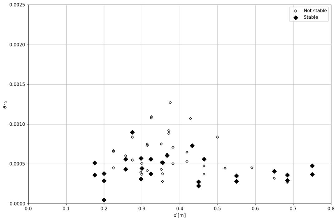
Figure E.4: Data points from the experimental wave flume tests showing the trend between the  $\theta_s$ -value and the water depth  $d$  in meters using the spectral velocity determination
