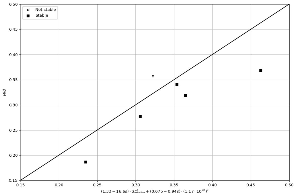
Figure G.2: Relation of the resulting stability function for the pink reef including data points, with the unstable points above the line and stable points below
