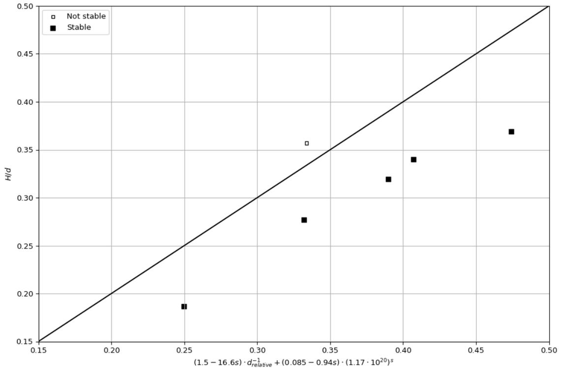
Figure G.7: Relation of the resulting stability function for the 2x2 reef including data points, with the unstable points above the line and stable points below
