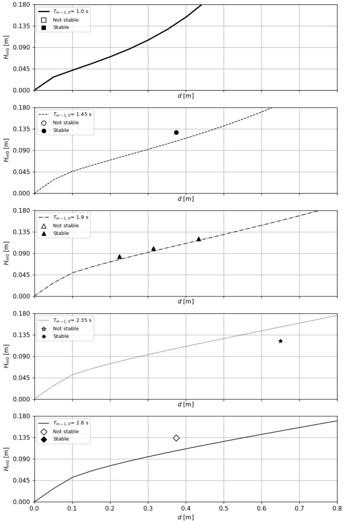
Figure G.3: Separate plots for the relation between the significant wave height and the water depth for several spectral periods for the double plate (pink) reef model according to the Morison stability prediction, including the data points of the flume tests
