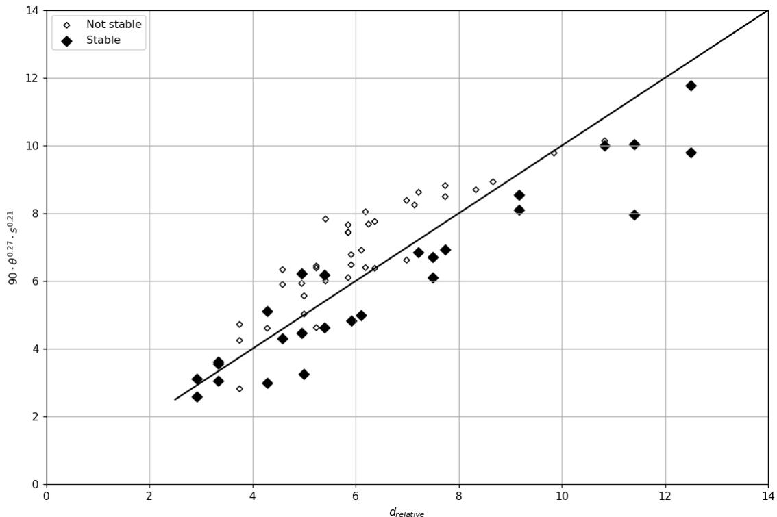
Figure 4.10: Relation of the prediction method using the mobility parameter for the single plate (grey) reef with data points, with most of the unstable points above the line and stable points below
