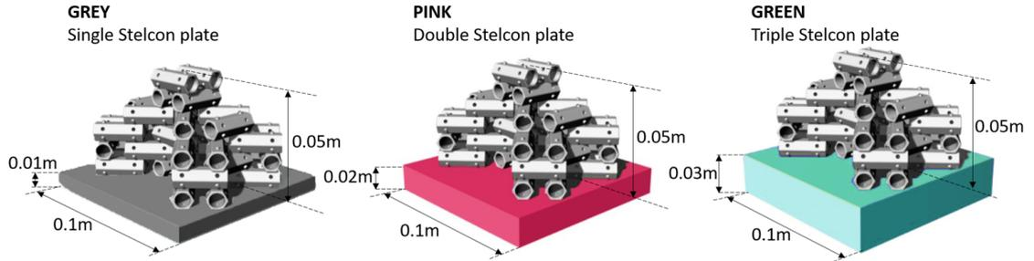
Figure 3.5: Schematic of the models of the reefs, with a single (left), double (middle), or triple (right) layer of Stelcon concrete plates
