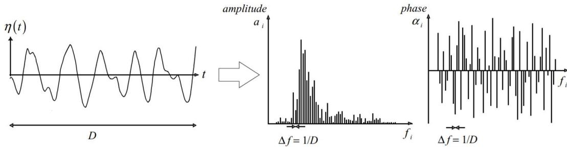
Figure 2.2: Observed surface elevation for a duration  $D$  and the corresponding amplitude and phase spectrum (Holthuijsen, 2007)
