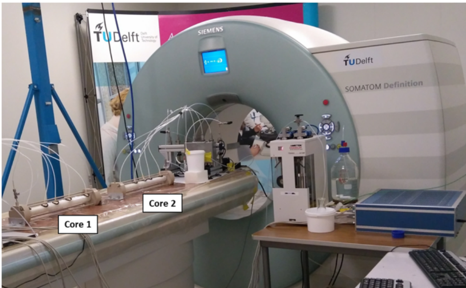
Figure 3.5: Computed Tomography (CT) Scanner, in this photograph set up for two cores.
