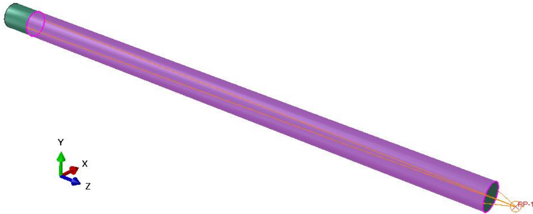
Figure 4.17: Example of a coupling between a reference point (red) and a section of a part (pink).
