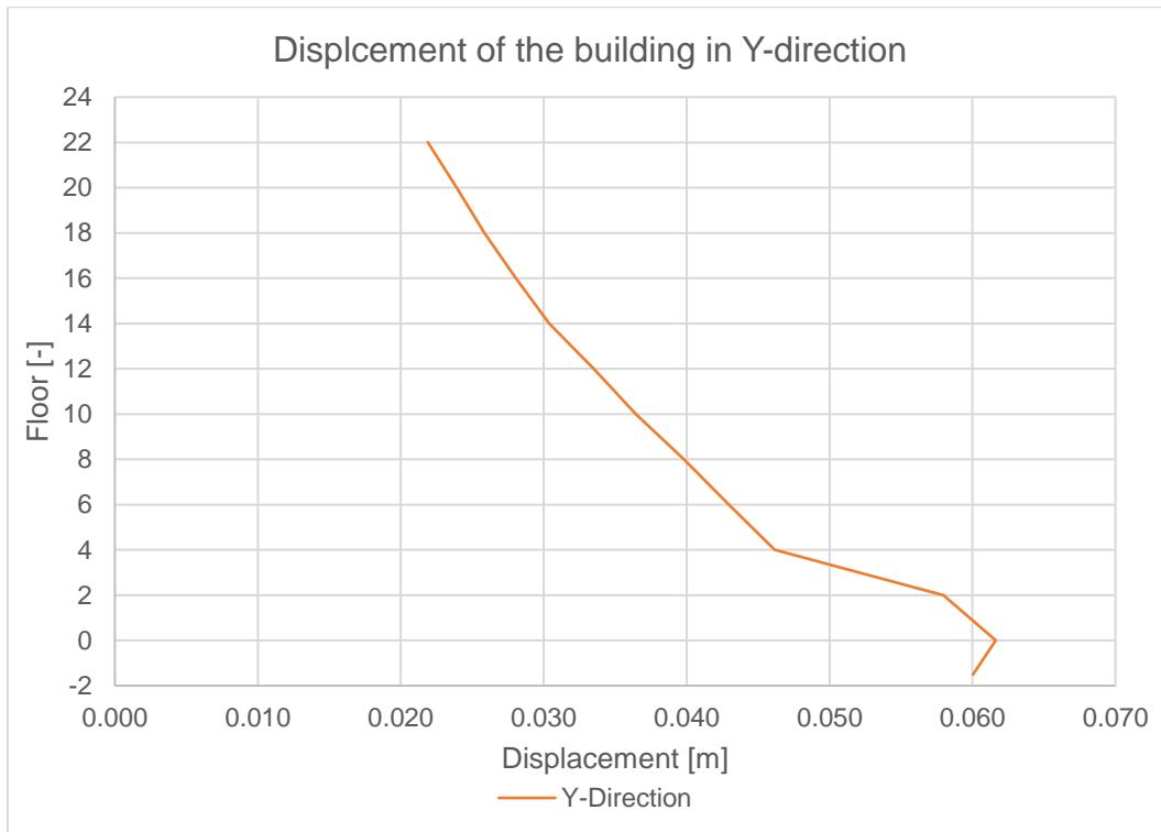
Figure 6.5: Displacement of each floor in Y-direction at t=2.88 seconds, plotted over the height of the building.
