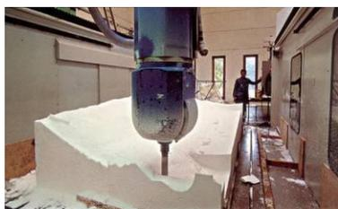
(a): CNC milled formwork
