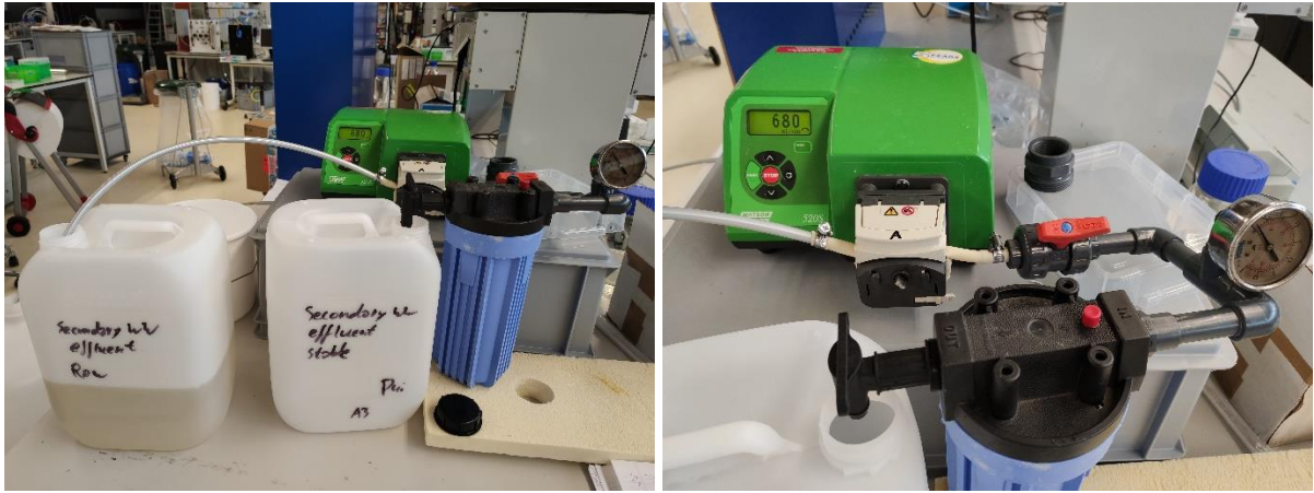
Figure 14 Microfiltration setup front view (left) and top view (right). The blue holder contains the filter cartridge and a pressure meter is at the feed flow. The green apparatus is the peristaltic pump.
