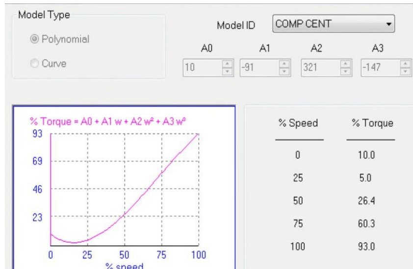
Figure 3-14: The Load Curve Fitting of Typical Industrial Rotary Pump
