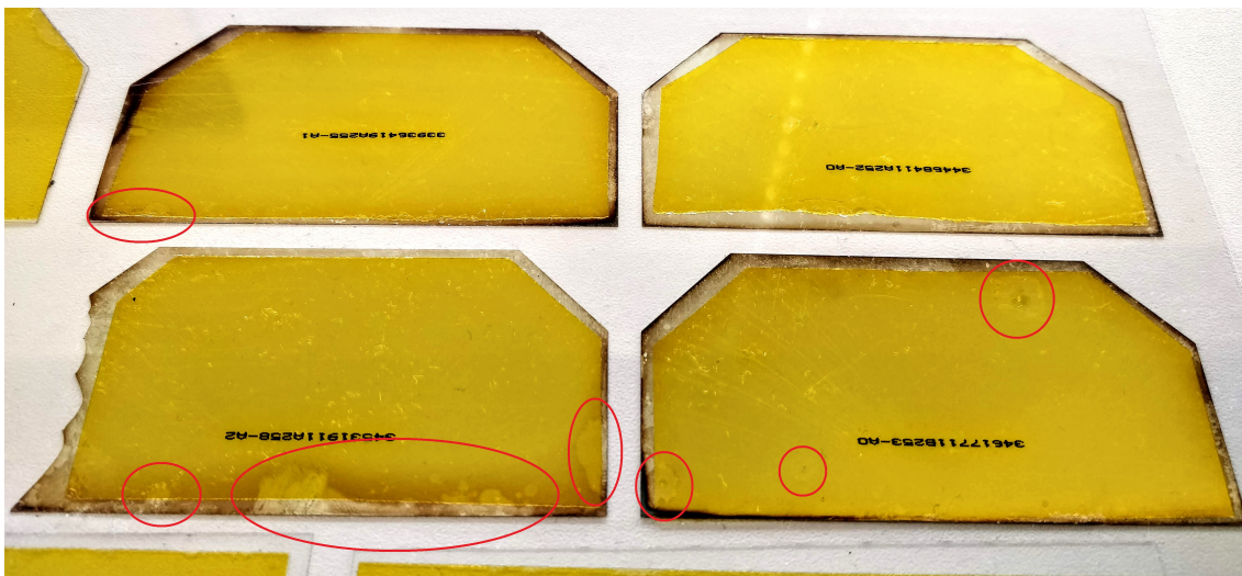
Figure 4.9: Air bubbles are visible under the double-sided tape between the solar cells and the plastic sheet.
