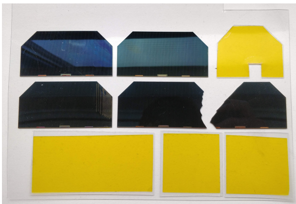
Figure 4.7: All tests performed on a see-through plastic sheet to verify the use of double-sided tape to bond solar cells to a PCB.
