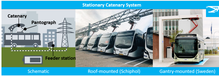
FIGURE 1 Schematic view of stationary catenary charging for bus [18][15][17]
