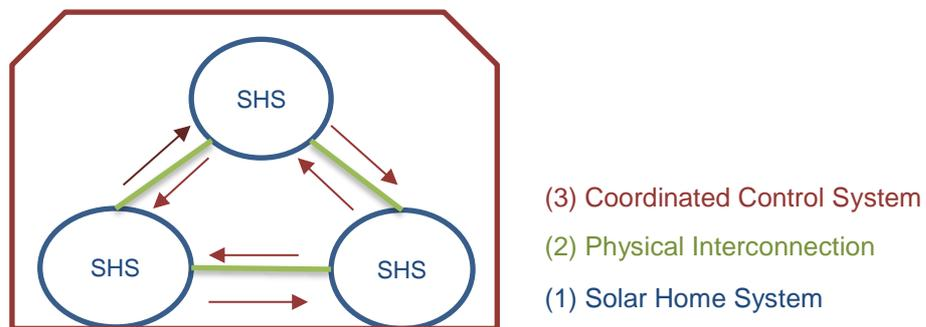
**Figure 2-5 Bottom-up Approach for LVDC Forming**
