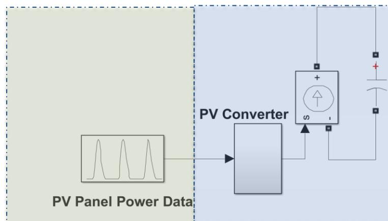
**Figure 3-7 PV Generator Block Model**
