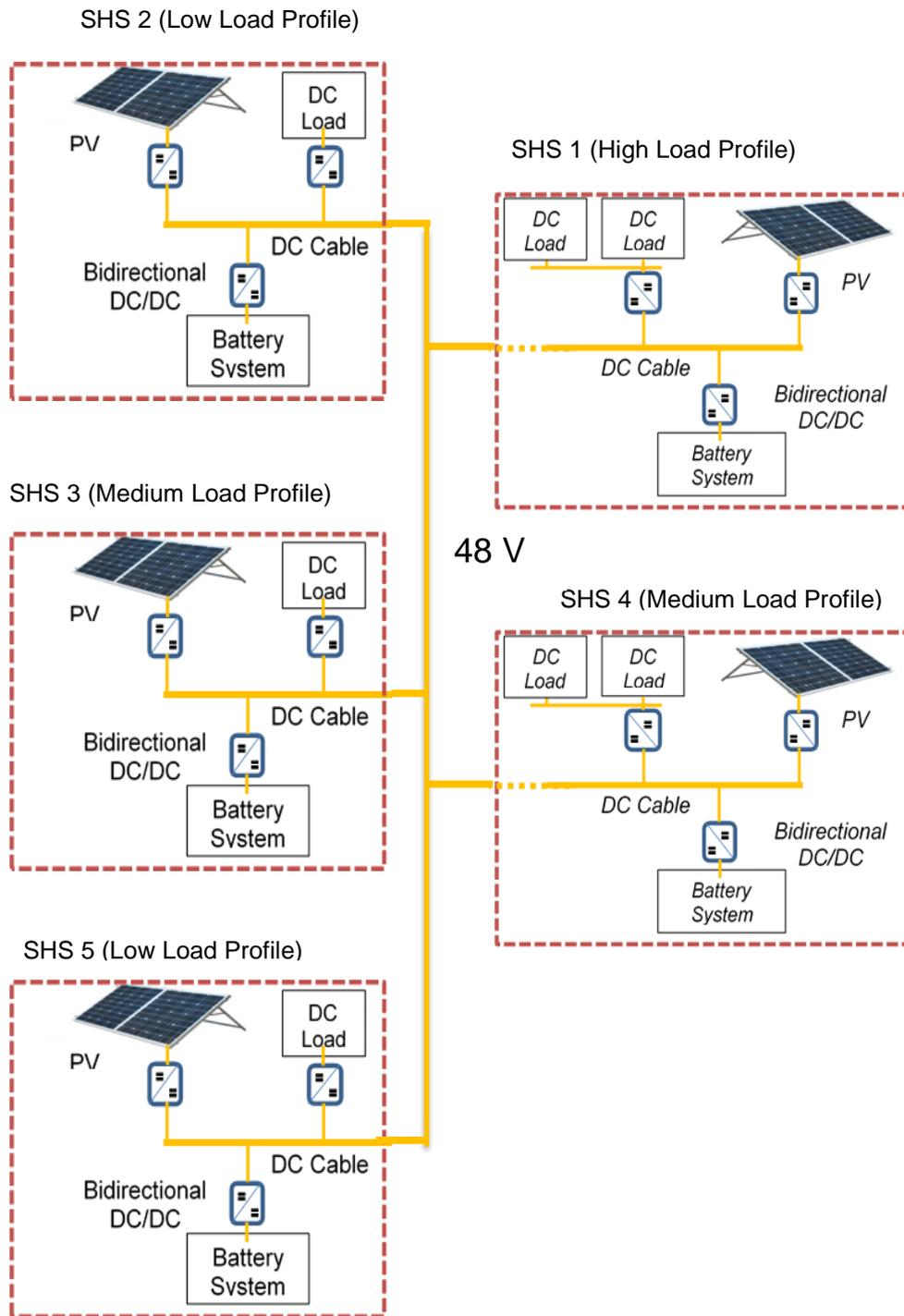
Figure 4-2 Interconnection Topology in 48V
