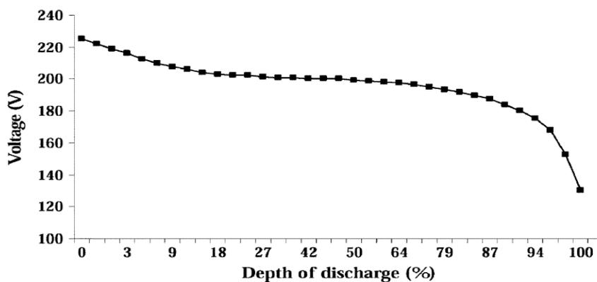
**Figure 3-9 Depth of Discharge Characteristic of Battery [32]**
