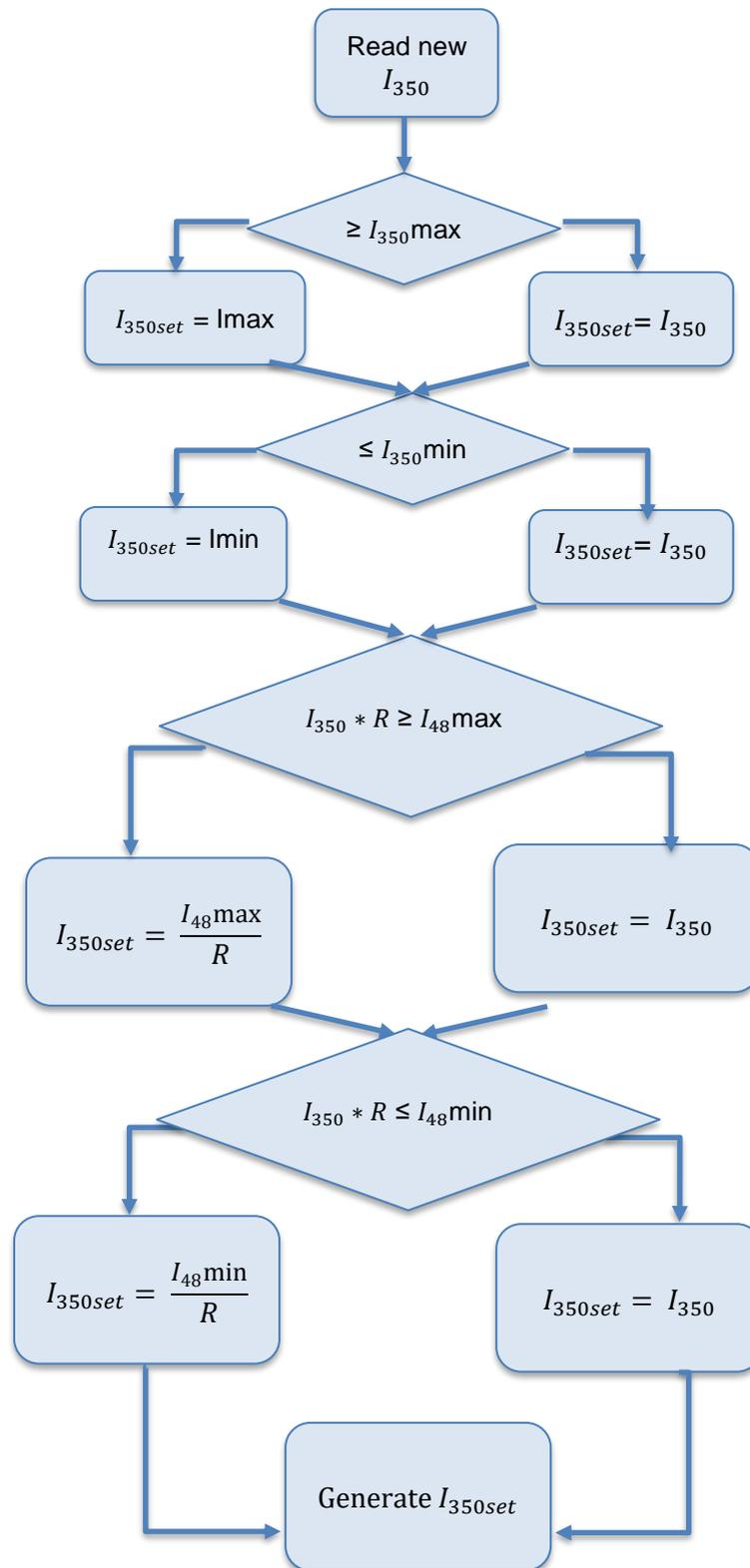
**Figure 4-14 Current output limit check**
