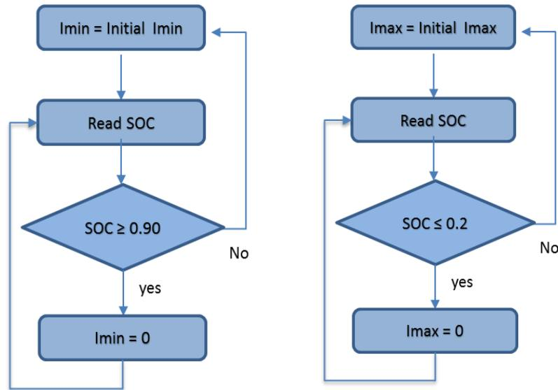
**Figure 3-21 (a) Current Absorbing Limiter (b) Current Injection Limiter**
