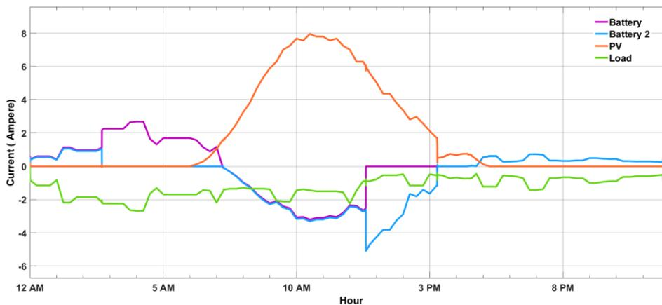
**Figure 3-33 Current Characteristic of Multiple Batteries**
