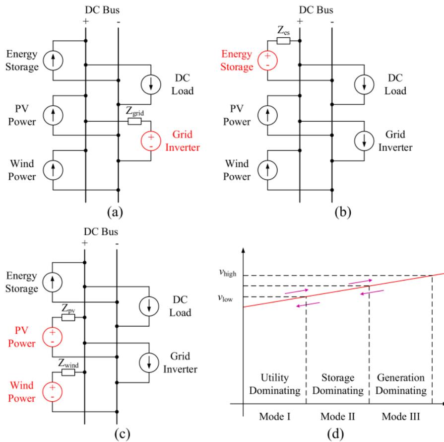
**Figure 2-12 (a) Utility Dominating Mode (b) Storage Dominating Mode (c) Generation Dominating Mode (d) Operation Mode Selection [24]**
