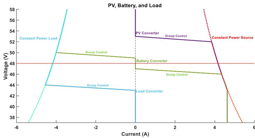
Figure 3-16 Converter Operation Modes
