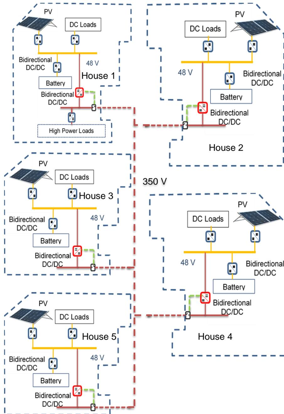
Figure 4-11 Interconnection Topology in 350V
