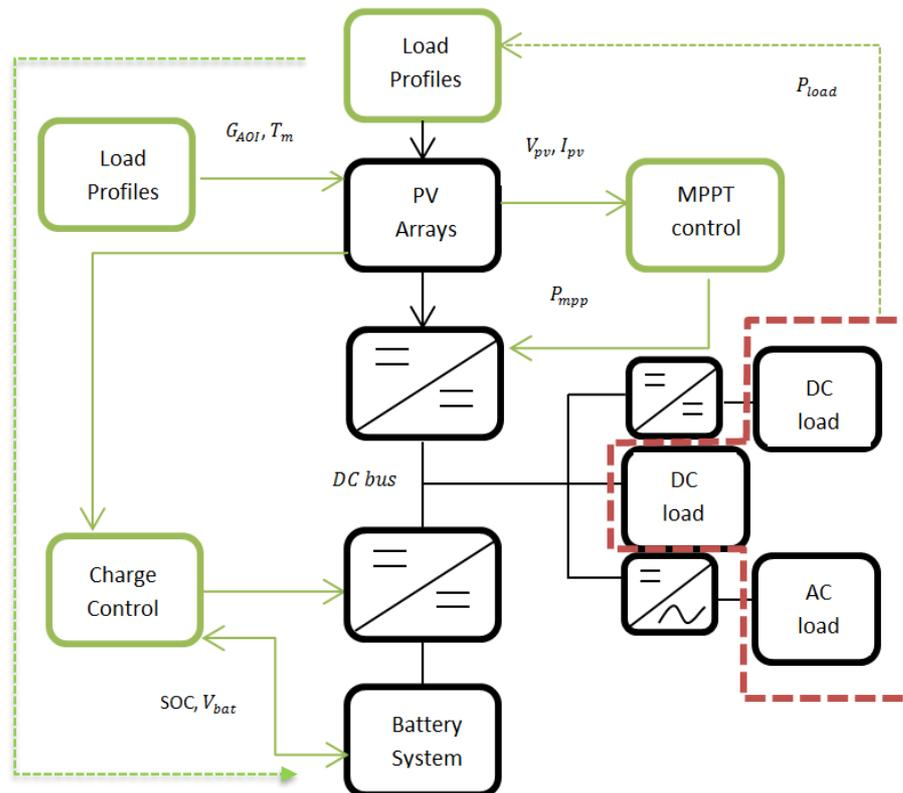
Figure 3-1 Solar Home System Modelling Workflow
