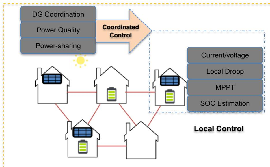
**Figure 2-6 Multilevel Control Scheme**
