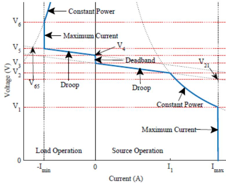
Figure 3-15 Voltage Set Points for Different Operation Modes [38]
