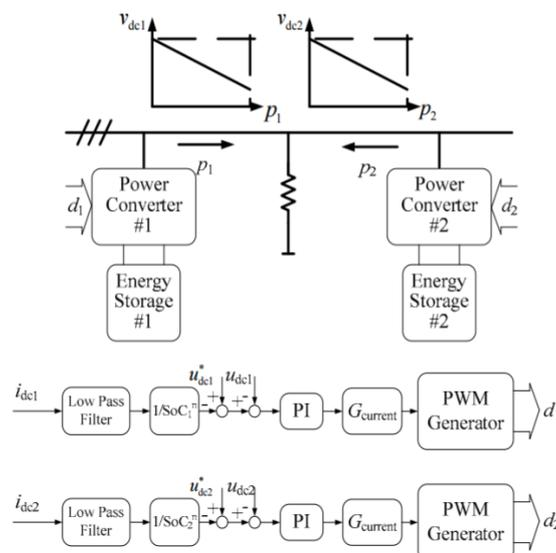
**Figure 2-9 Modified Droop Control Based on SOC [25]**
