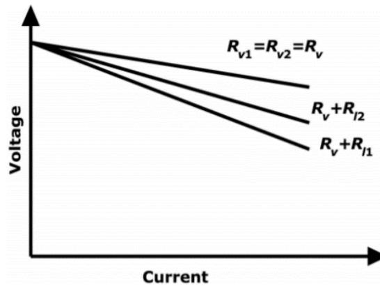
**Figure 2-11 Effect of Line Resistances on Droop Gain [29]**
