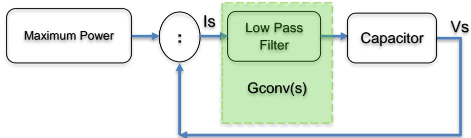
**Figure 3-18 Constant Power Controlled Models**
