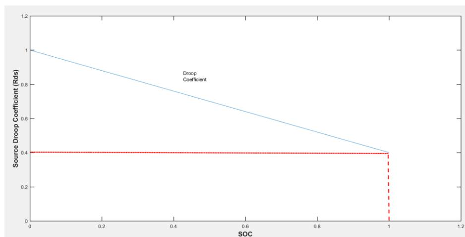
**Figure 3-24 Linear Discharging Droop Multiplication Factor**
