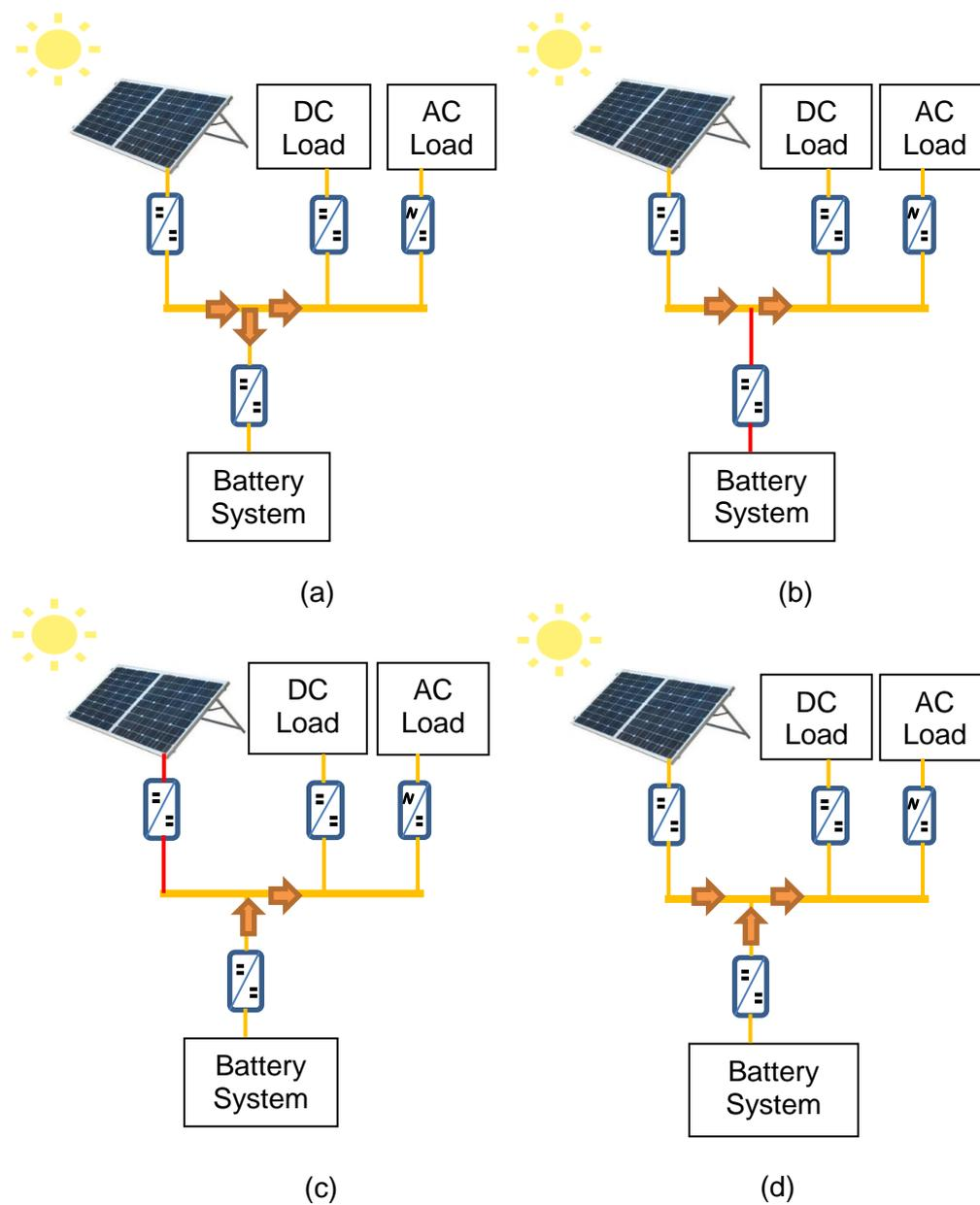
**Figure 3-12 Power Flow in SHS**
