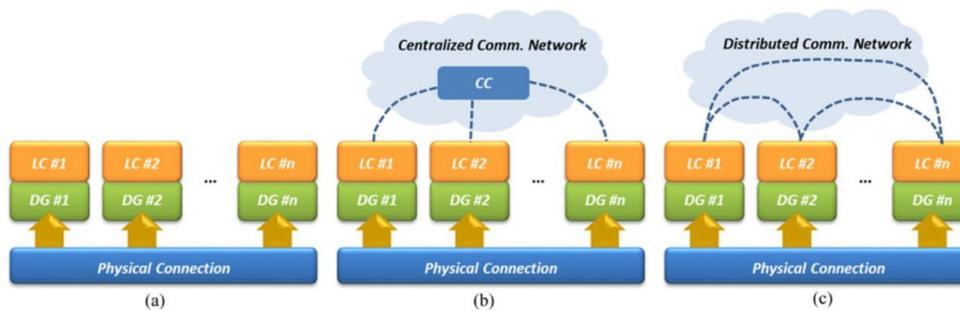
**Figure 2-7 (a) Decentralized Control, (b) Centralized Control, (c) Distributed Control [23]**
