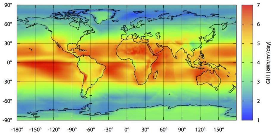
**Figure 3-8 Equivalent Sun Hours of The World based on Average Global Horizontal Irradiance [30]**
