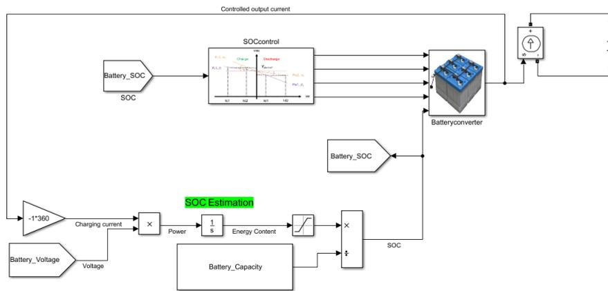
**Figure 3-10 Battery Model**
