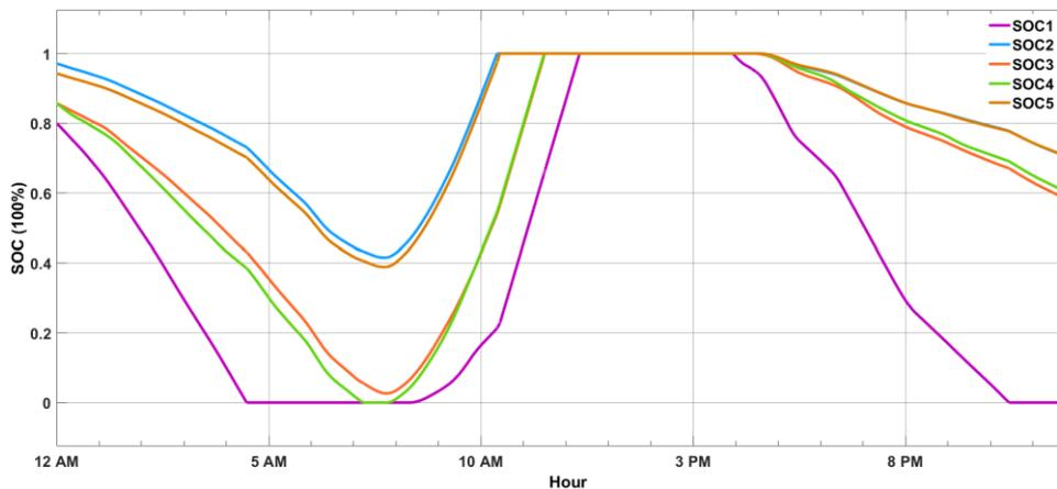
**Figure 4-10 SOC of Batteries in the Interconnected Houses**
