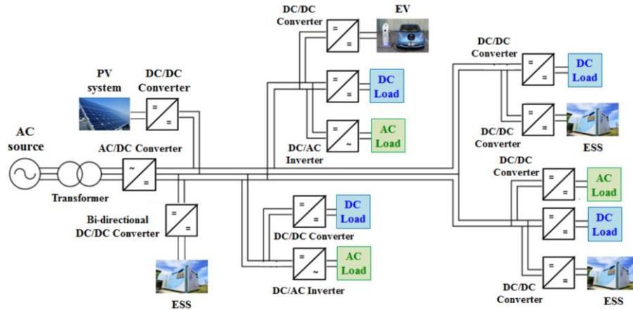
**Figure 2-4 Low Voltage Direct Current Distribution Network [21]**
