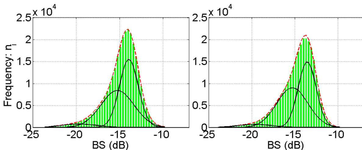
**Fig 2.** Histogram (light bar) of averaged (over small surface patches) backscatter data corrected for local slopes, its three Gaussians (solid line), and its best fit (dashed line) at angle  $\theta = 60^\circ$  over the whole area; left transducer (left); right transducer (right); number of Gaussian PDFs  $r = 3$ .
