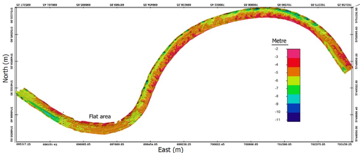
**Fig. 1** Bathymetry map of river Waal, the Netherlands; Km 876–886 (close to Nijmegen).
