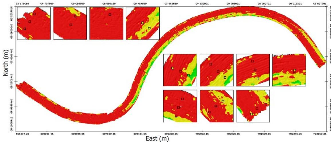
**Fig 3.** Acoustic classification map of Waal river (Km 876–886) obtained from backscatter data at  $\theta = 64, 62, \dots, 20^\circ$ . For each angle separate classification has been applied and results put in a single map. The frames indicate a zoom-in of classification results for areas where grab samples have been taken.
